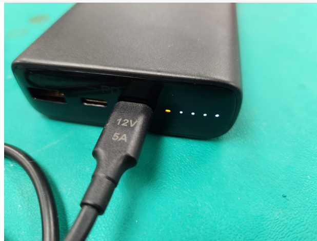
Figure 12. Connect the calibration Y-cable to an external battery pack using the USB-C connection.
