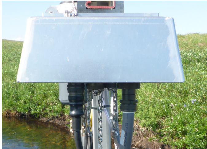
Figure 67. Reconnect sensor and ethernet cables to Grape.
