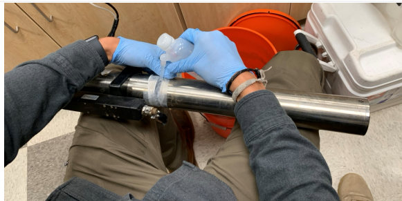
Figure 23. Fill Optical Area with Equilibrated DI Water.
