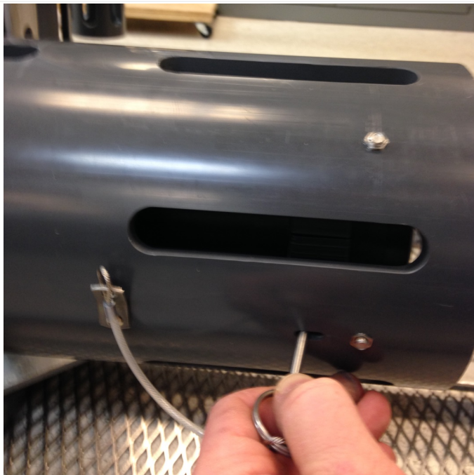
Figure 64. Pull 4 lock pins to remove captive discs.
