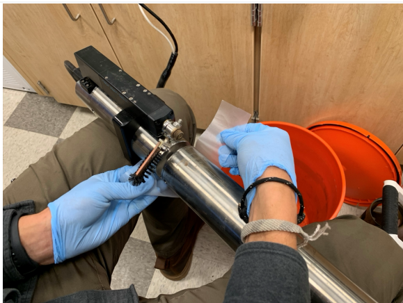
Figure 21. Cut Parafilm to Size.
