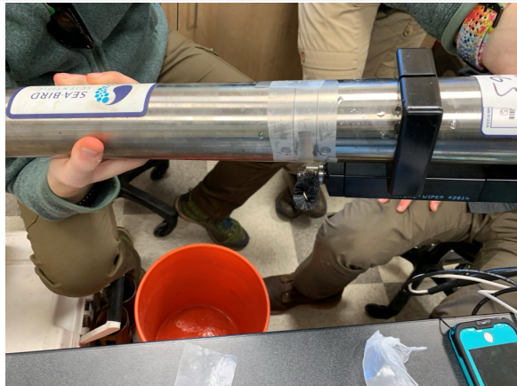
Figure 22. Wrap Parafilm around Optical Area of SUNA.
