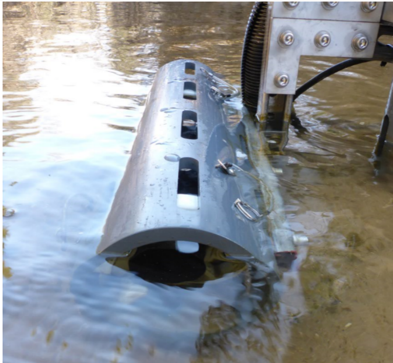
Figure 55. SUNA Partially Submerged in Stream.
