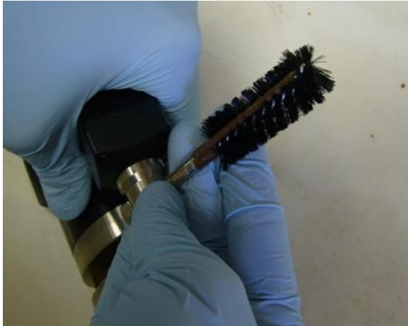
Figure 20. Physically Move Wiper on SUNA.
