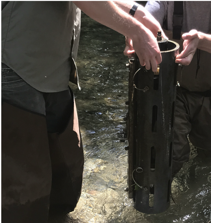
Figure 62. Remove SUNA PVC enclosure.
