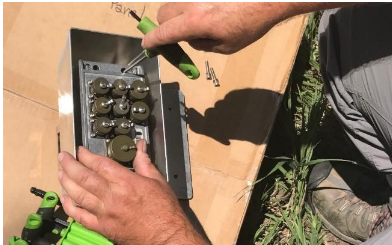
Figure 10. Remove Grape from Grape Shields (D06 KING)
