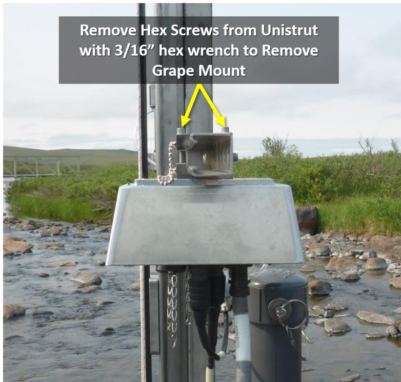
Figure 11. Remove Grape Shield with 3/16" Hex Wrench
