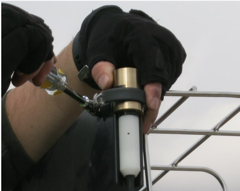
Figure 21. Secure Sensor in Mount
