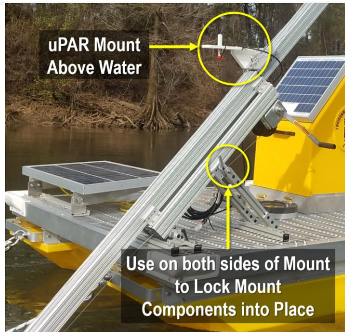
Figure 25. uPAR Mount Locking Mechanism Example
