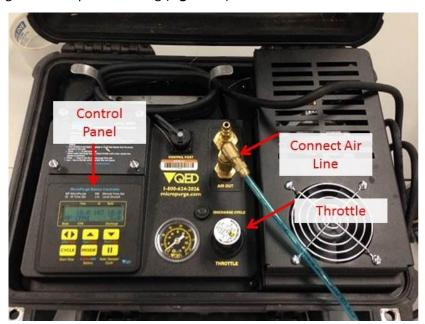
Figure 21. Attach blue air-line to controller.
