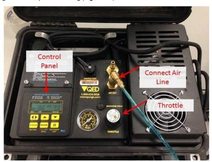
Figure 21. Attach blue air-line to controller.
