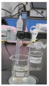
**Figure 39.** Image of titration set-up with digital titrator, stir bar, pH meter and temperature probe. Ensure nothing is touching the sides and bottom of the beaker or the stir bar
