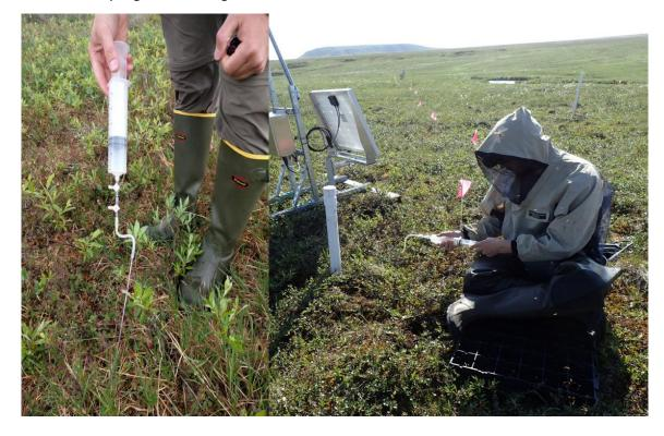
Figure 28. Sampling needle and syringe setup.
