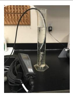
Figure 23. Groundwater Chemistry Collection cell using a 1000 mL graduated cylinder.
