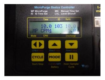
Figure 24. Groundwater pump control panel screen. Note the Refill and Discharge times on the right.
