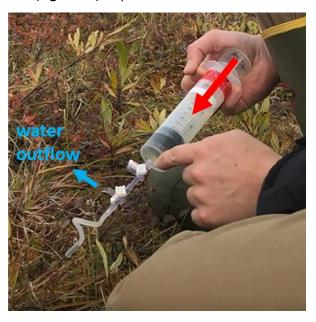
Figure 30. Stopcock position for expelling water during bubble-free sampling.
