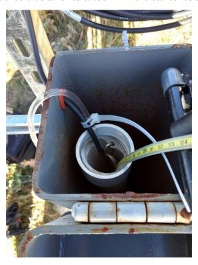
Figure 25. Pump tubing secured in place with zip tie.
