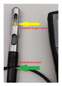
Figure 10. Picture of handheld meter showing location of sensors on probe.
