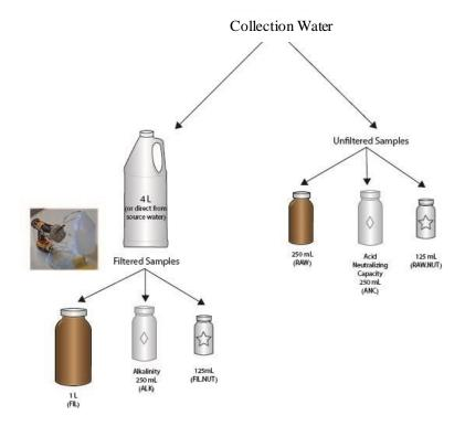
**Figure 6**. Flowchart of Water Chemistry Sample Collection and Filtration. à Indicates 250 mL, wide-mouth sample bottles that remain at the Domain Support Facility for titration analysis. ☆ Indicates 250 mL, wide-mouth sample bottles that are frozen (-20°C) immediately prior to shipping. ANC is only collected monthly. Letters in parenthesis indicate the sample type that correspond to the chemistry labels (see Figure 8).
