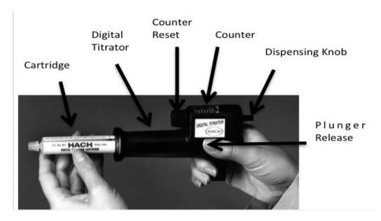
Figure 39. Inserting titrant cartridge into digital titrator. Photo from the Hach Digital titrator manual.
