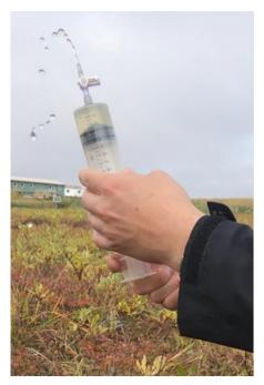
Figure 31. Expel air bubbles from the syringe during bubble-free sampling.
