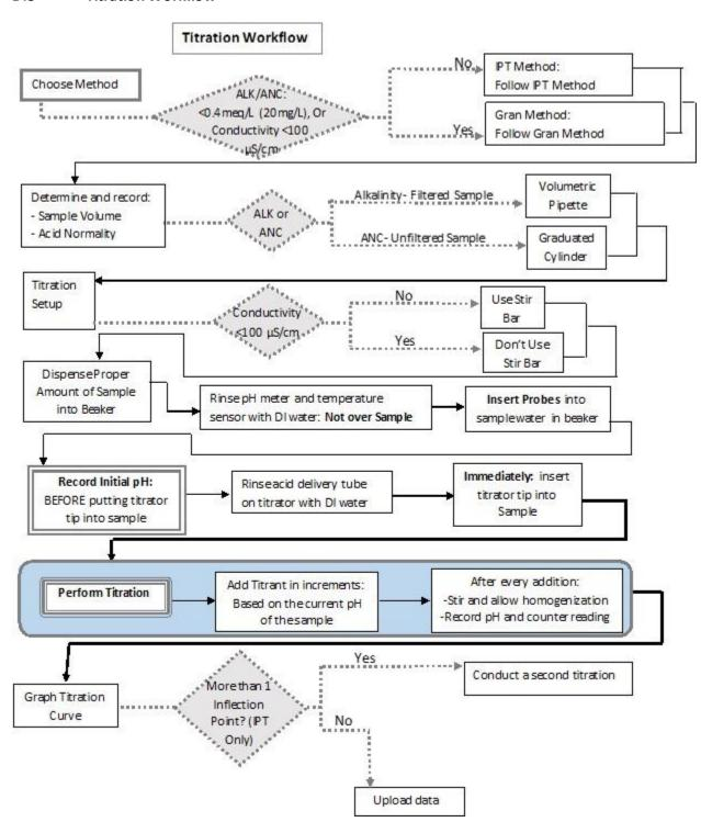
Figure 38. High Level titration workflow.
