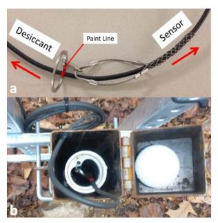
**Figure 14**. Correct cable position for groundwater sensors. a) Cable paint should align with the metal docking ring. b) The metal docking ring should sit flush within the PVC collar.
