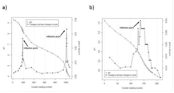
**Figure 42**. Example of inflection point titration using a digital titrator of a) a high alkalinity sample and b) a low alkalinity sample. Note difference in Y-axis scale. (Modified from USGS TWRI Book 9, Alkalinity, Version 3.0 7/2006).
