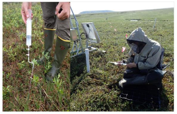
Figure 30. Sampling needle and syringe setup.
