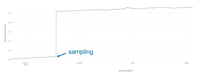
Figure 43. Example of a large jump in LO pressure data after a sampling event.
