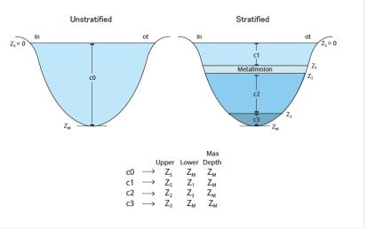
**Figure 12**. Example of an unstratified and stratified lake water column a) sampling depths with placement of thermocline and b) identification of upper and lower section depths. In deep lakes, 2 thermal stratifications may occur, creating 3 sections. Note, hypolimnion sampling is determined by the hypolimnion section depth (i.e., thickness). If hypolimnion thickness is < 4m, collect one sample at midpoint of hypolimnion. If hypolimnion thickness is > 4m collect an integrated sample.
