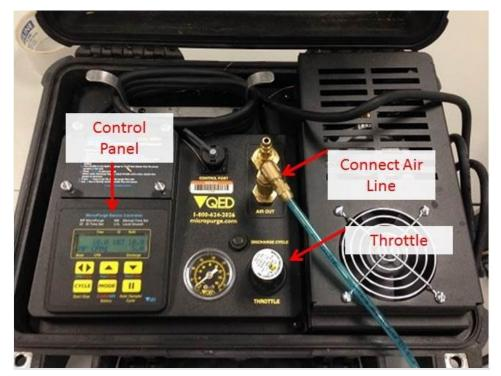
Figure 23. Attach blue air-line to controller.
