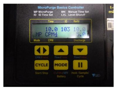
Figure 26. Groundwater pump control panel screen. Note the Refill and Discharge times on the right.
