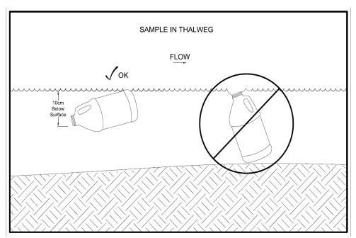
Figure 11. Diagram of proper and poor placement of a water sample bottle.
