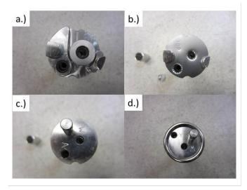
**Figure 19**. Assembly of the fitting plate at the top of the pump for holding the air and water lines. (a) Bare top of pump. (b) Fitting/grab plate added ("TOP" must face upwards). (c) Top plate added. (d) Collar added to lock parts (a-c) together.
