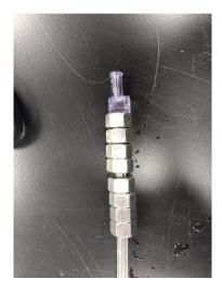
Figure 27. Nuts added to peristaltic pump tubing for weight.
