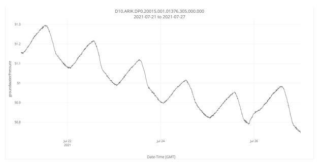
**Figure 15**. DQ Blizzard plot for groundwater pressure for an individual wellowera 1-week period. Pressure is roughly 51 kPa indicating that there is about 5.1 m of water above the sensor. If the sensor is 0.5m from the well bottom, then the water column height is roughly 5.6m.
