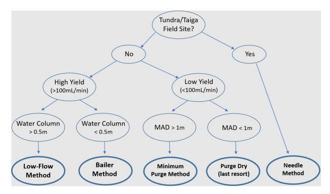
**Figure 16**. Decision tree for determining appropriate groundwater sampling method.
