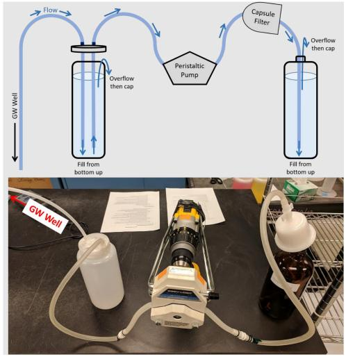
**Figure 33**. Filtering setup to minimize sample aeration during filtration for low-flow groundwater samples.
