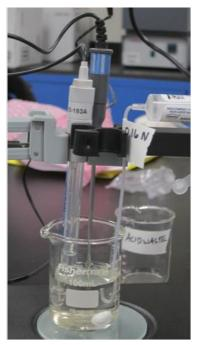
**Figure 41**. Image of titration set-up with digital titrator, stir bar, pH meter and temperature probe. Ensure nothing is touching the sides and bottom of the beaker or the stir bar
