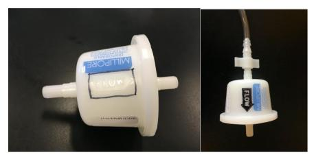
**Figure 36**. Pictures highlighting flow arrow on capsule filter. These have been highlighted for the purpose of the picture but will not be on your filter. They can be hard to see. Ensure you set up the filter so water flows through it correctly, with the flat end at the end of the setup.
