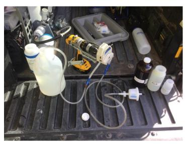
**Figure 35**. Pump and filter setup, including a peristaltic sampling pump (modified from Woessner 2007), a 4 L sample bottle, tubing connectors to connect peristaltic and C-flex tubing, and a capsule filter.
