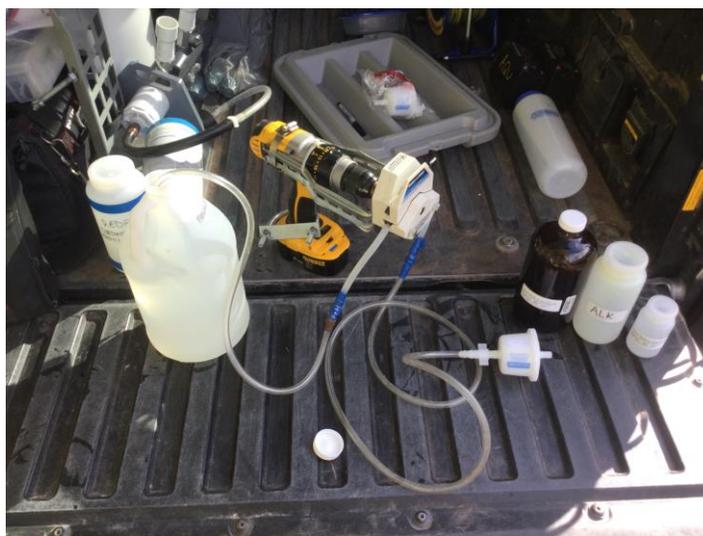
**Figure 34.** Pump and filter setup, including a peristaltic sampling pump (modified from Woessner 2007), a 4 L sample bottle, tubing connectors to connect peristaltic and C-flex tubing, and a capsule filter.
