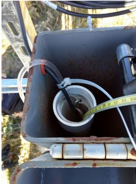
Figure 27. Pump tubing secured in place with zip tie.
