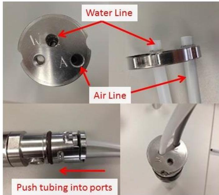
**Figure 20.** Attaching grey air-line and white water-lines to pump (top-right photo shows lines pushed through top plate and “teeth” of grab plate).
