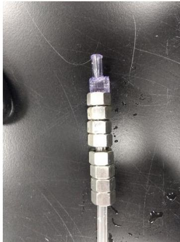
Figure 26. Nuts added to peristaltic pump tubing for weight.
