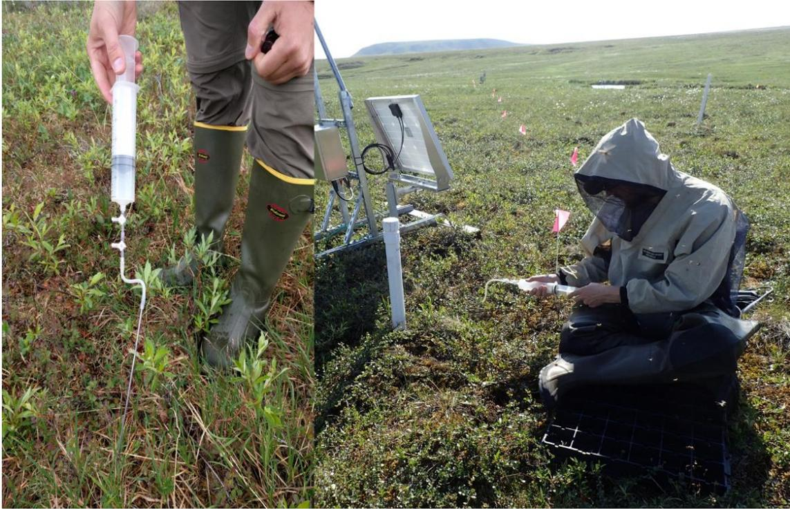
**Figure 29.** Sampling needle and syringe setup.
