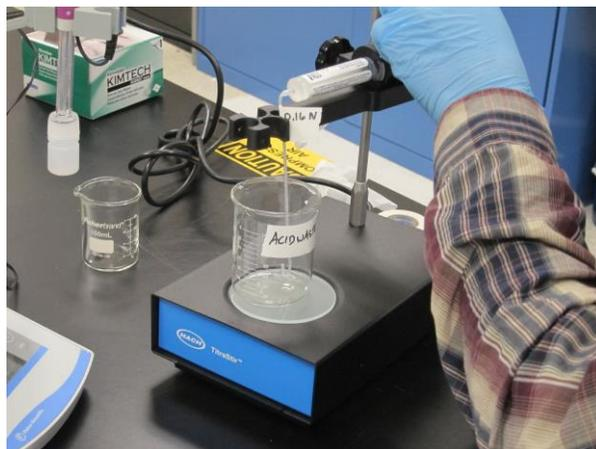
**Figure 39.** Diagram of procedure to expel acid from digital titrator set-up into a temporary acid waste container.
