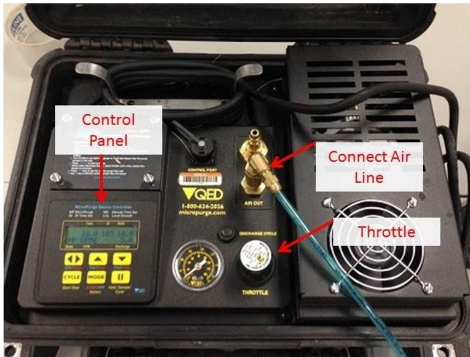
Figure 22. Attach blue air-line to controller.
