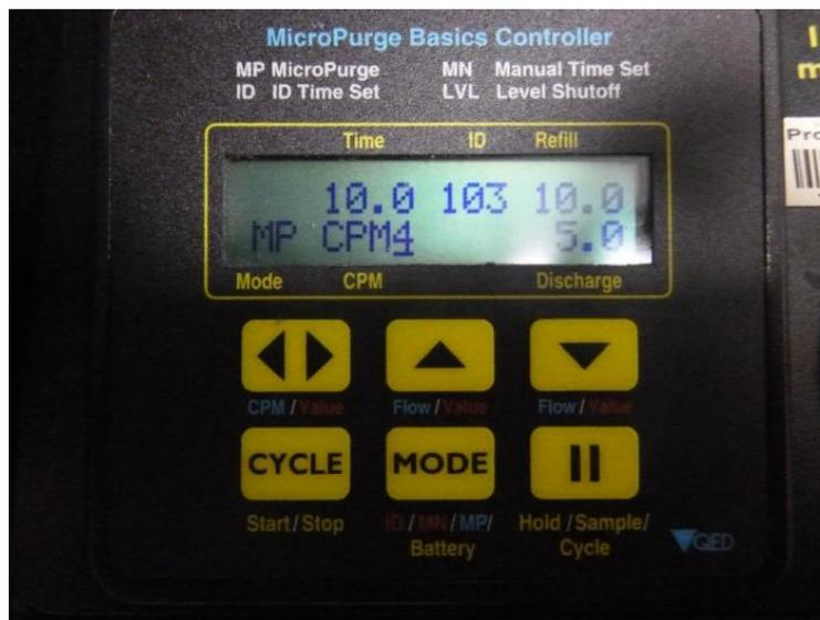
**Figure 25.** Groundwater pump control panel screen. Note the Refill and Discharge times on the right.
