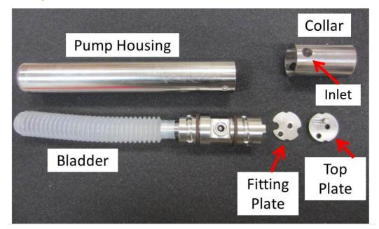
Figure. Components of the sampling pump.
