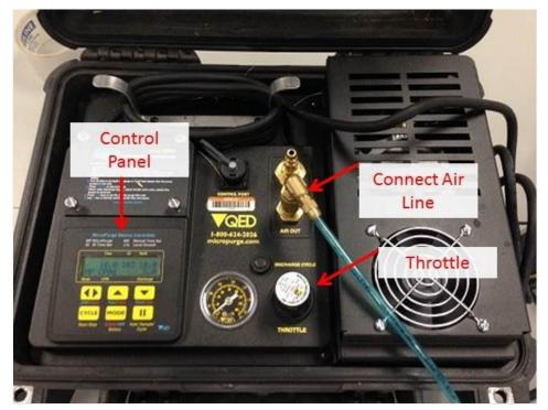
Figure 22. Attach blue air-line to controller.
