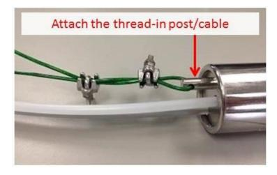
Figure 21. Attach post and cable to the pump via the top plate.
