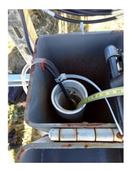
Figure 27. Pump tubing secured in place with zip tie.
