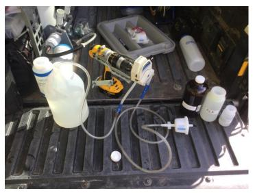
**Figure 34**. Pump and filter setup, including a peristaltic sampling pump (modified from Woessner 2007), a 4 L sample bottle, tubing connectors to connect peristaltic and C-flex tubing, and a capsule filter.
