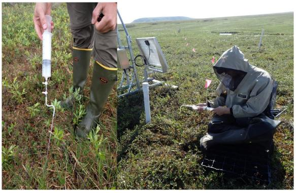
Figure 29. Sampling needle and syringe setup.
