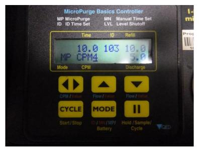
Figure 25. Groundwater pump control panel screen. Note the Refill and Discharge times on the right.
