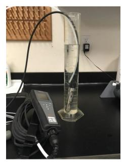
Figure 24. Groundwater Chemistry Collection cell using a 1000 mL graduated cylinder.
