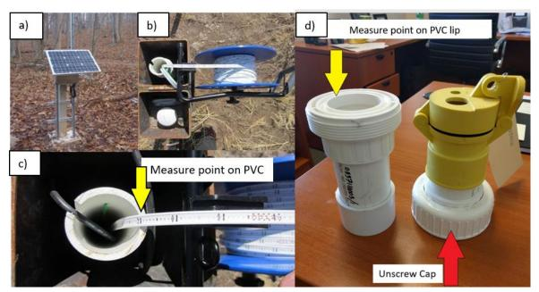
**Figure 18**. Groundwater well depth measurements (a) Standard groundwater well at a NEON site (b) Water-level tape attached to outer well casing. (c) Reading the depth to water from the water-level tape on standard well. The tapes are marked in "meters" with each foot increment marked in red. Readings are taken at the top of the inner PVC casing. (d) Cap disconnection and measurement point for wells with snorkel cap design.
