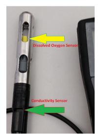
Figure 10. Picture of handheld meter showing location of sensors on probe.
