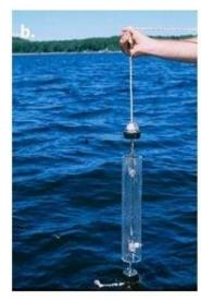
**Figure 13**. Illustration of Kemmerer sampler for water sampling (a). Illustration of how the Kemmerer is lowered into the water by holding the rope and messenger (b)
