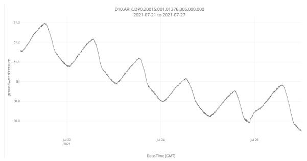
**Figure 15**. DQ Blizzard plot for groundwater pressure for an individual well over a 1-week period. Pressure is roughly 51 kPa indicating that there is about 5.1 m of water above the sensor. If the sensor is 0.5m from the well bottom, then the water column height is roughly 5.6m.
