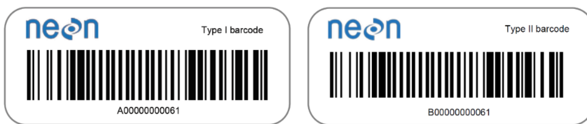
Figure 7. An example of a Type I and Type II barcode. These large-size, field-tolerant barcodes have a prefix of 'A' (Type I) and B (Type II) followed by 11 numbers.
