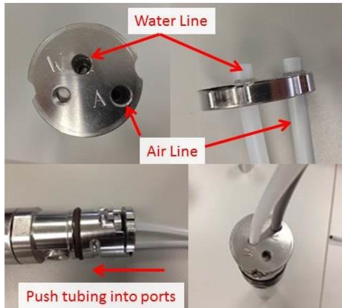
Figure 21. Attaching grey air-line and white water-lines to pump (top-right photo shows lines pushed through top plate and “teeth” of grab plate).
