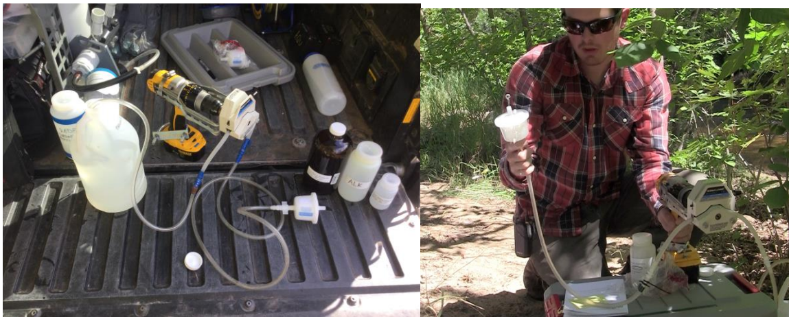
Figure 34. Pump and filter setup, including a peristaltic sampling pump (modified from Woessner 2007), a 4 L sample bottle, tubing connectors to connect peristaltic and C-flex tubing, and a capsule filter. Image on right shows the correct way to prime the filter by holding it upright.
