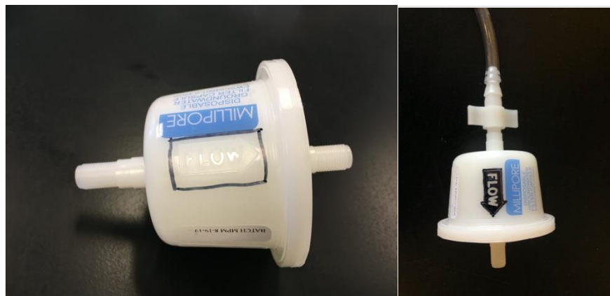
Figure 35. Pictures highlighting flow arrow on capsule filter. These have been highlighted for the purpose of the picture but will not be on your filter. They can be hard to see. Ensure you set up the filter so water flows through it correctly, with the flat end at the end of the setup.
