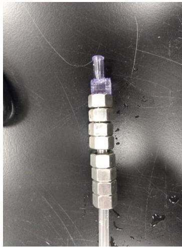
Figure 27. Nuts added to peristaltic pump tubing for weight.
