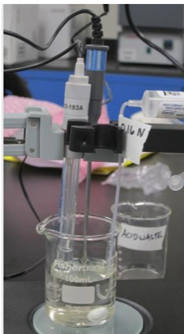
Figure 40. Image of titration set-up with digital titrator, stir bar, pH meter and temperature probe. Ensure nothing is touching the sides and bottom of the beaker or the stir bar.
