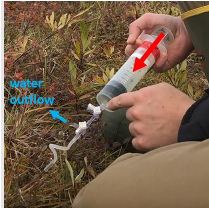
Figure 31. Stopcock position for expelling water during bubble-free sampling.
