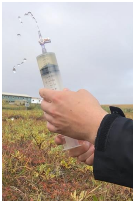
Figure 30. Expel air bubbles from the syringe during bubble-free sampling.
