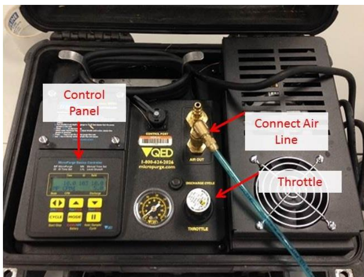
Figure 23. Attach blue air-line to controller.
