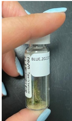
Figure 23. Photo of CN vial with human readable label and Type IV barcode.
