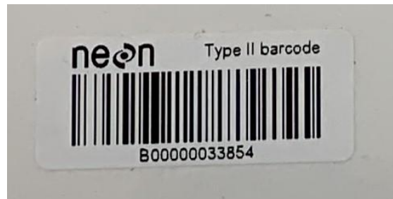
Figure 11. An example of a Type II barcode. These large-size, freeze-tolerant barcodes have a prefix of 'B' followed by 11 numbers.
