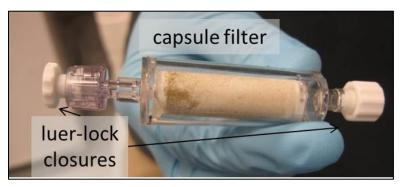
Figure 10. Capsule (Sterivex®) filter and luer lock closures
