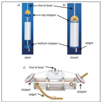
**Figure 6.** Vertical Kemmerer water sampler in the a) open or cocked position and b) closed (after dropping the messenger) position. c) Horizontal Van Dorn in the open position.
