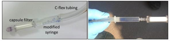
**Figure 2**. Filter adapter for peristaltic pump, you may put the C-flex tubing inside or outside (cut off top) of the 3 mL syringe.
