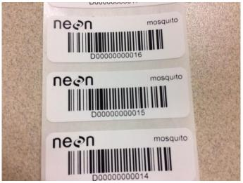
Figure 5. Example of adhesive barcode labels.
