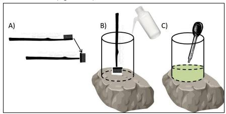
**Figure 13.** Schematic of PVC periphyton sampler. A) Cut off the head of a toothbrush, and re-adhere it horizontally. B) Set the PVC sampler on the substrate, and scrub the substrate surface using the modified toothbrush. Rinse rock surface. C) Remove water + algae sample with a turkey baster or disposable pipet.
