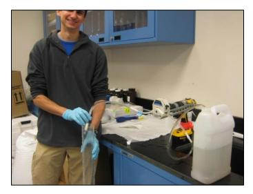
**Figure 12**. Pump sample water out of the 4-gallon HDPE jug, through the peristaltic pump, the through the Sterivex® filter, and into a graduated cylinder to measure the volume filtered.
