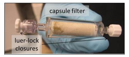
Figure 13. Capsule (Sterivex®) filter and luer lock closures.
