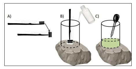
**Figure 17**. Schematic of PVC periphyton sampler. A) Cut off the head of a toothbrush and re-adhere it horizontally. B) Set the PVC sampler on the substrate and scrub the substrate surface using the modified toothbrush. Rinse rock surface. C) Remove water + algae sample with a turkey baster or disposable pipet.
