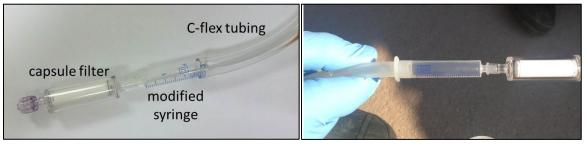
**Figure 4**. Filter adapter for peristaltic pump, you may put the C-flex tubing inside or outside (cut off top) of the 3 mL syringe.
