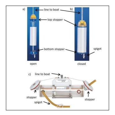
**Figure 9**. Vertical Kemmerer water sampler in the a) open or cocked position and b) closed (after dropping the messenger) position. c) Horizontal Van Dorn in the open position.
