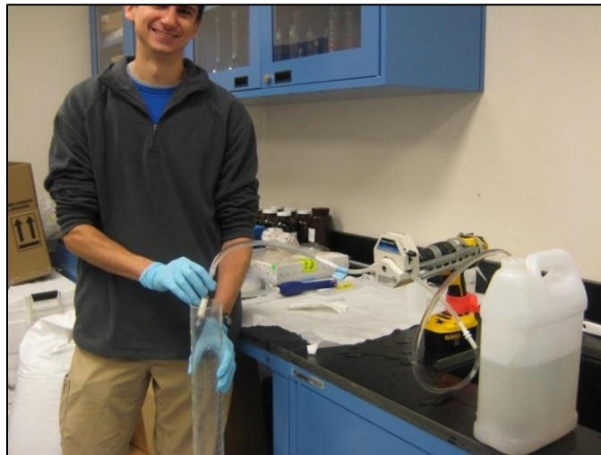
Figure 12. Pump sample water out of the 4-gallon HDPE jug, through the peristaltic pump, the through the Sterivex filter, and into a graduated cylinder to measure the volume filtered.
