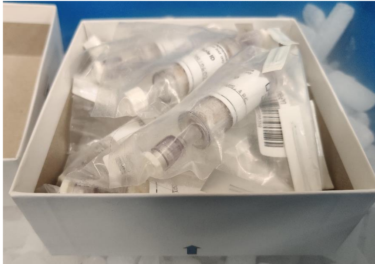
Figure 20. Cryogenic storage box for ARC samples. Use these boxes rather than zip-top bags for shipping to the Biorepository.
