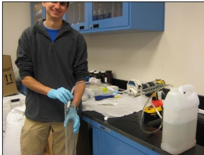
Figure 11. Pump sample water out of the 4-gallon HDPE jug, through the peristaltic pump, the through the Sterivex filter, and into a graduated cylinder to measure the volume filtered.
