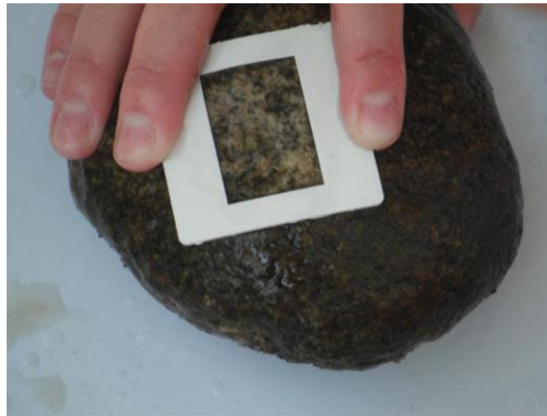
Figure 20. Template placement for epilithon protocol. (Note: Samples should not be processed in direct sunlight.)
