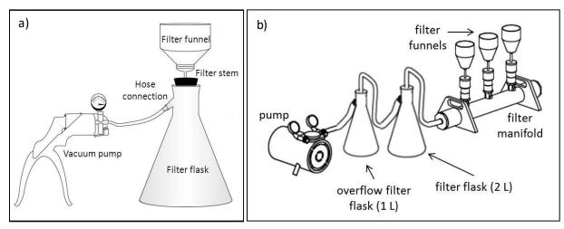
Figure 39. Filter apparatus setup: a) hand pump; b) filter manifold.
