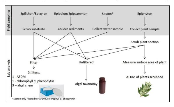
Figure 36. Lab schematic diagram for all aquatic sites.
