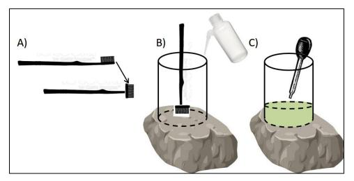
**Figure 26.** Schematic of PVC periphyton sampler. A) Cut off the head of a toothbrush, and re-adhere it horizontally using epoxy. B) Set the PVC sampler on the substrate, and scrub the substrate surface using the modified toothbrush. Rinse rock surface. C) Remove water + algae sample with a turkey baster or disposable pipet.
