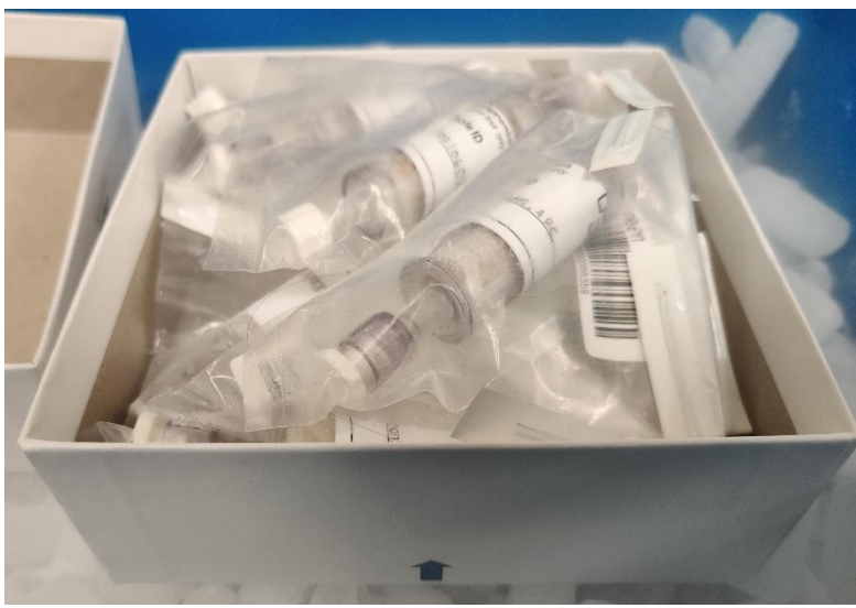
Figure 36. Cryogenic storage box and Whirl-Paks for ARC samples. Apply human readable labels to the filter capsule and the barcode inside the Whirl-Pak. Use these boxes rather than zip-top bags for shipping to the Biorepository.
