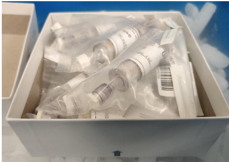
Figure 36. Cryogenic storage box and Whirl-Paks for ARC samples. Apply human readable labels to the filter capsule and the barcode inside the Whirl-Pak. Use these boxes for shipping to the Biorepository.
