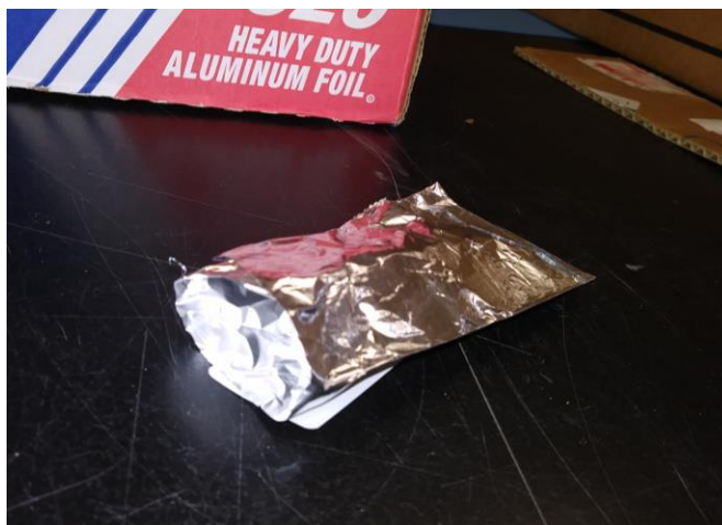
Figure 42. Example of a filter packet left slightly open for drying algal chemistry filters in the drying oven.
