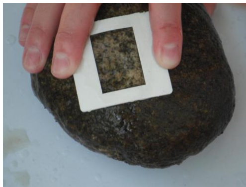
Figure 26. Template placement for epilithon protocol. (Note: Samples should not be processed in direct sunlight)
