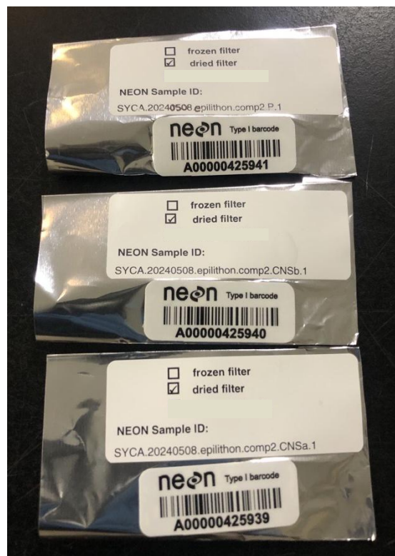
Figure 36. Example of algal chemistry packets with human readable label and barcode label.
