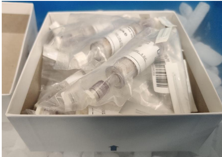
Figure 37. Cryogenic storage box and Whirl-Paks for ARC samples. Apply human readable labels to the filter capsule and the barcode inside the Whirl-Pak. Use these boxes for shipping to the Biorepository.
