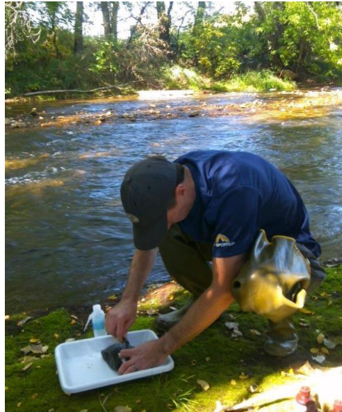
Figure 25. Process samples on the stream bank, out of direct sunlight.
