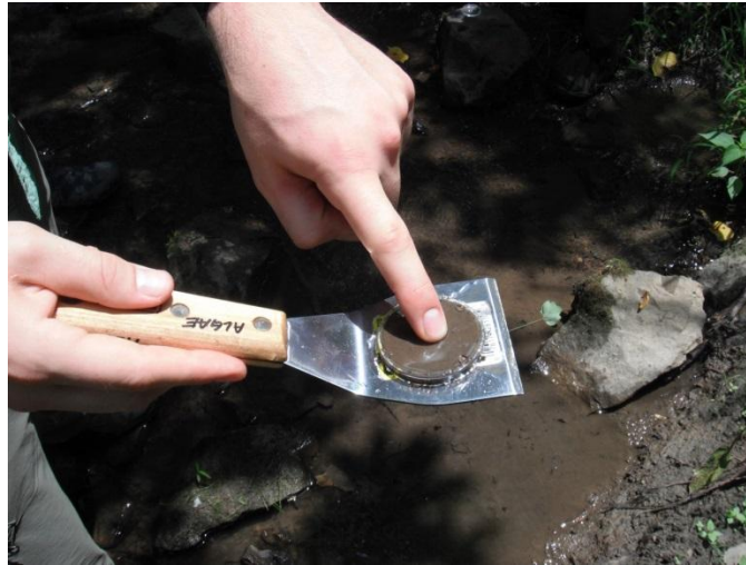
Figure 30. An epipelton sample collected with the Petri dish lid and metal spatula (NOTE: gloves must be worn when sampling).
