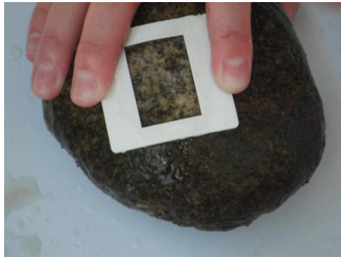
Figure 26. Template placement for epilithon protocol. (Note: Samples should not be processed in direct sunlight)
