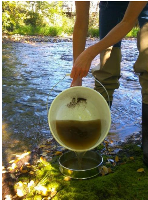
Figure 36. Carefully pours water from the 3 gallon bucket into the sieve.
