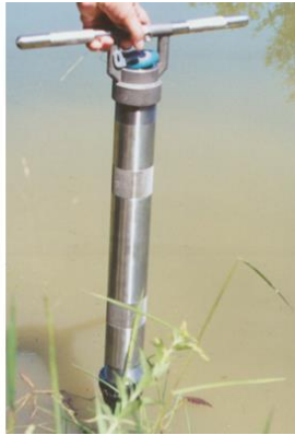
Figure 25. Push the hand corer through the water and into the sediments at a 90° angle
