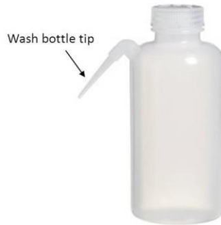
Figure 23. Removing the tip of the 500 mL wash bottle helps makes rinsing easier and increases water pressure. This tip pulls easily out of the main body of the wash bottle.
