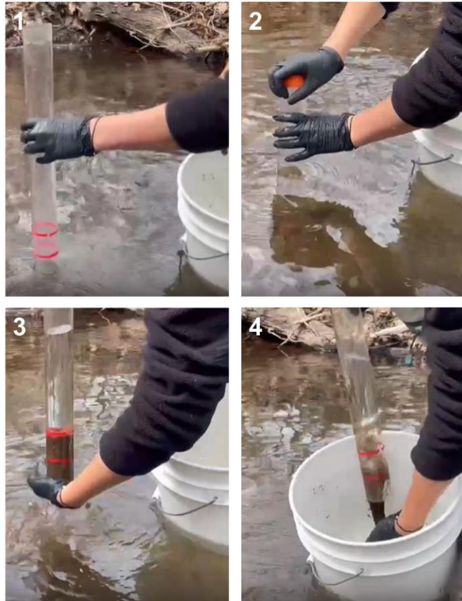
Figure 26. Steps for using the core liner tube alone. 1) Insert the liner tube into the sediments vertically; 2) Cap the liner; 3) Stop the bottom and pull the liner tube out of the sediments; 4) Deposit sample material into the bucket.
