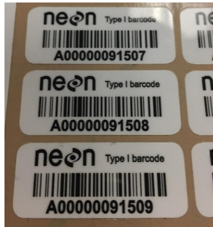
Figure 16. Example of adhesive barcode labels, Type I. These large-size, field-tolerant barcodes have a prefix of 'A' followed by 11 numbers.
