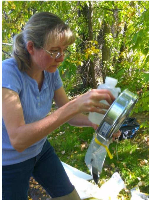
Figure 37. Rinse the sample from the sieve into the open container with the 500 mL wash bottle.
