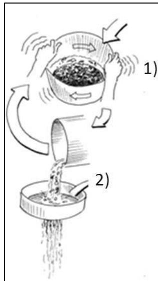
Figure 35. Process of elutriation (Dates and Byrne 1997).
