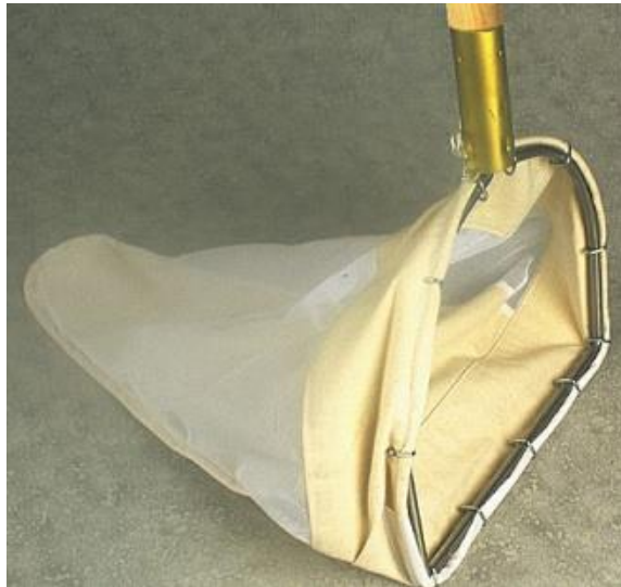
Figure 33. D-frame net, used for sweep samples in vegetation and silty habitats.
