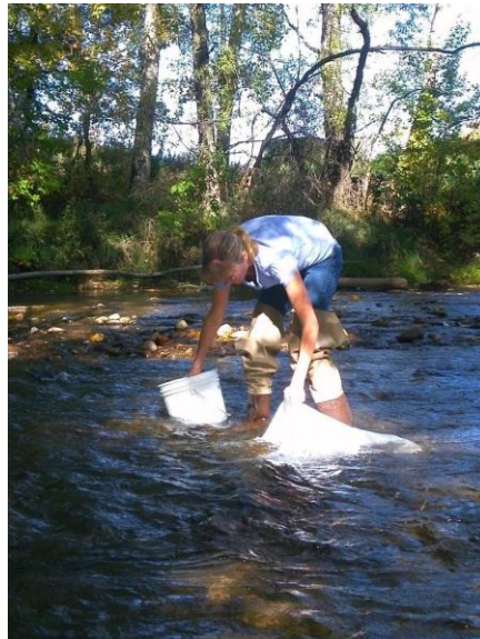
Figure 20. Hold the Surber net on the stream bottom, and keeps the bucket nearby for depositing rocks from the base of the Surber.
