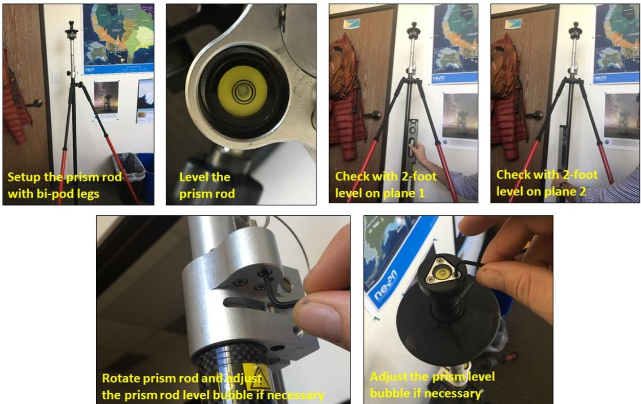
Figure 5. Calibrating the prism rod and prism head.
