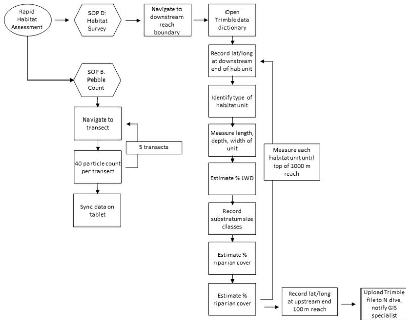
Figure 3. An expanded diagram of the workflow for the rapid habitat protocol.
