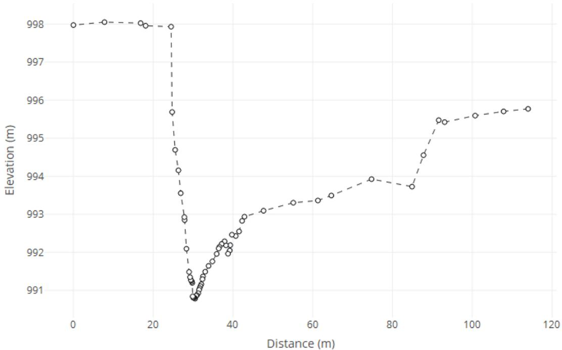
**Figure 15.** Example of high-resolution cross-section survey data where the floodplains, banks, and active channel are well-characterized by properly spaced points (each dot represents a mapped shot).
