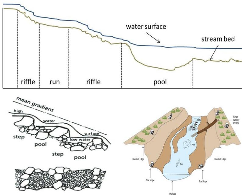
**Figure 17.** Above center: Long-profile illustration of riffle, runs, and pools. Bottom left: Illustration denoting step pools. Bottom right: Cross-section illustration denoting stream features.
