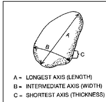
**Figure 18.** Illustration denoting the different substrate axes used during pebble count surveys.
