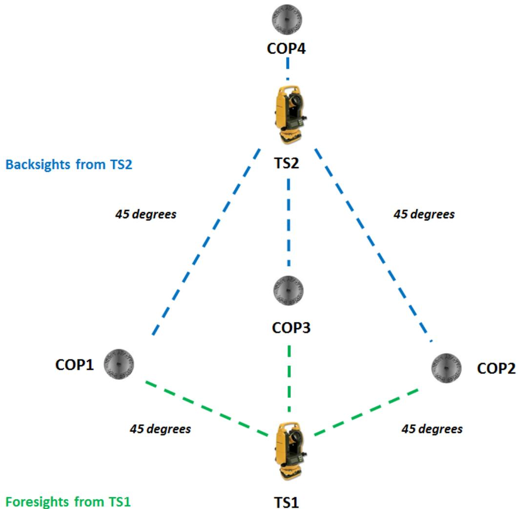
**Figure 13.** Idealized total station-control point setup using an optional fourth control point to set a second total station location (TS2).
