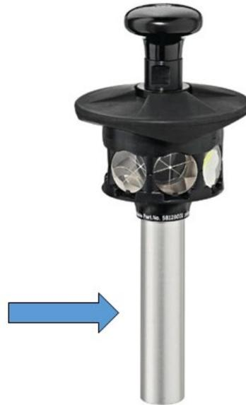
**Figure 4.** 10 cm pole segment (blue arrow) that connects the 360 degree prism (shown on the top of the segment) to the prism pole (not shown). This segment must always be installed during the stream morphology survey.
