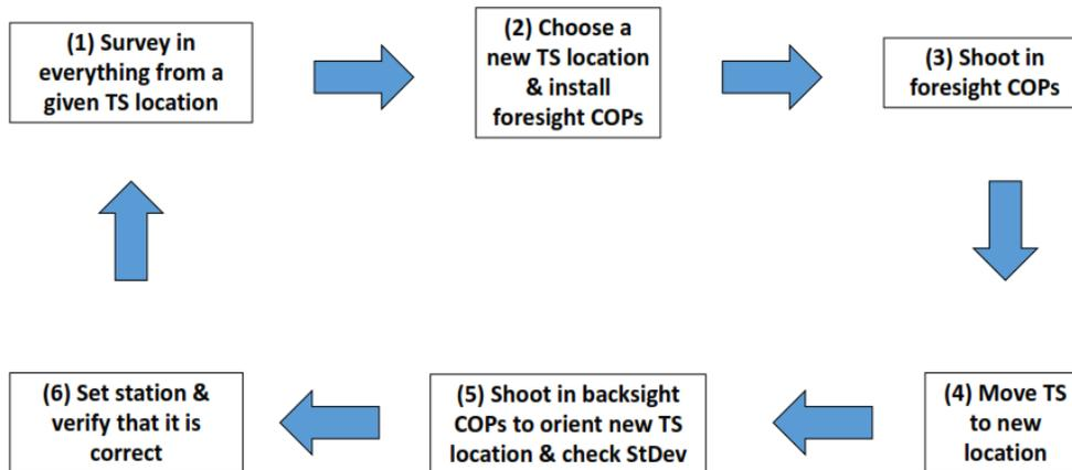
Figure 14. Total station setup workflow to be followed throughout the stream morphology survey.
