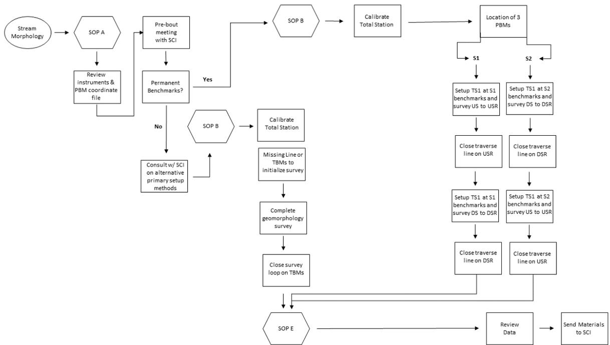
Figure 2. An expanded diagram of the workflow for the wadeable stream morphology protocol.
