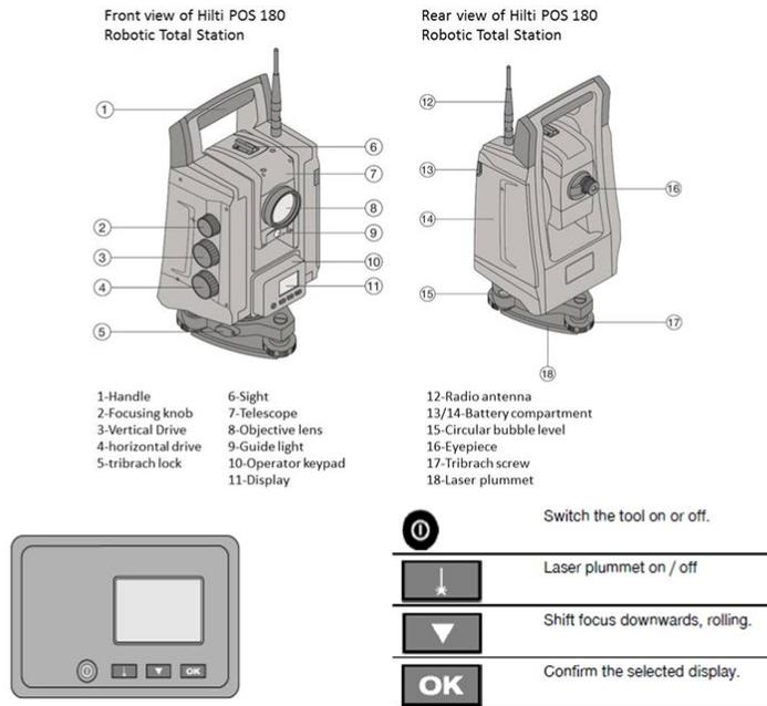
**Figure 6.** HILTI POS 180 Robotic Total Station schematics (above) and keypad diagram (below). Image credit: [www.us.hilti.com](http://www.us.hilti.com).
