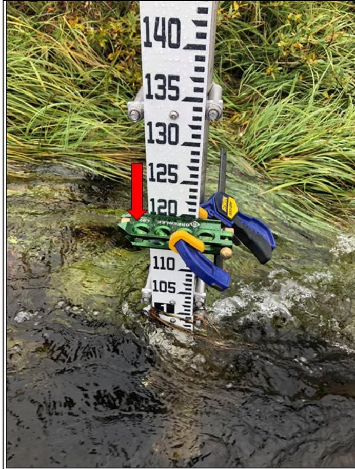
**Figure 16.** Mapping the staff gauge using a torpedo level and clamp. The red arrow indicates where the tip of the prism rod should be placed. The shot in this example would be coded “SP\_1.20M” as the tip of the prism rod is at exactly the 1.20 meter mark on the staff gauge.
