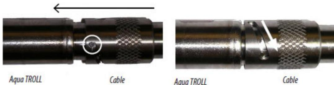
**Figure 18. Lock Cable with Pin and Slot**
