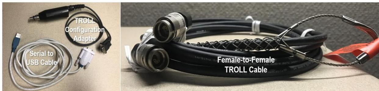
**Figure 79. Cables to Configure Aqua TROLLs**
