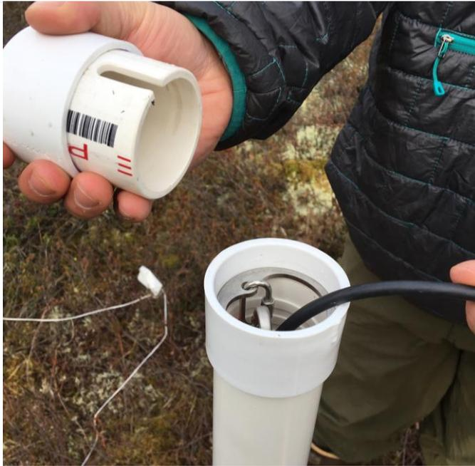
Figure 51. Remove PVC Cap from GWW (D19 CARI)
