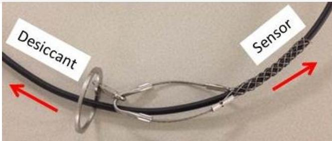
**Figure 56. Cable and Wire Basket with Well Dock Orientation**
