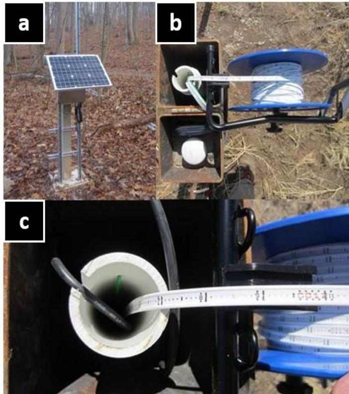
**Figure 23. (a) Standard groundwater well at a NEON site (b) Water-level tape attached to outer well casing. (c) Reading the depth to water from the water-level tape. The tapes are marked in “meters” with each foot increment marked in red.**
