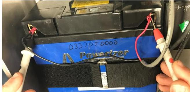
Figure 42. Use a DMM to Verify Battery Voltage
