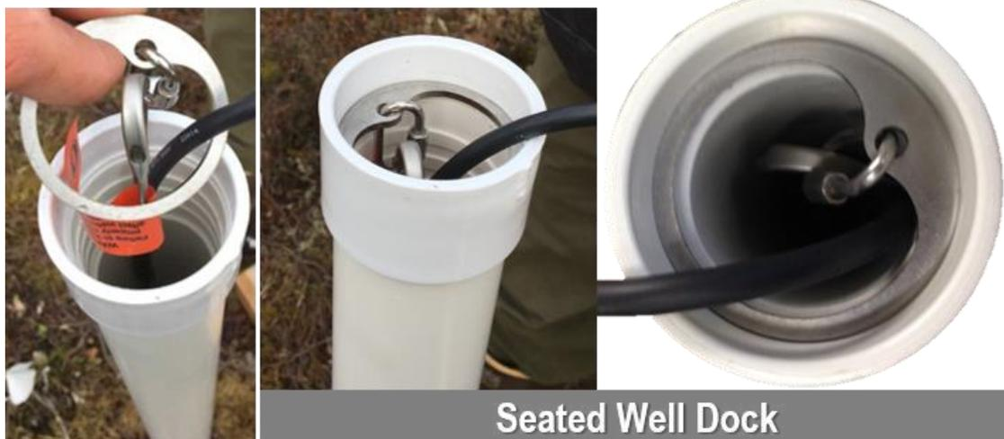
Figure 60. Well Dock in PVC casing
