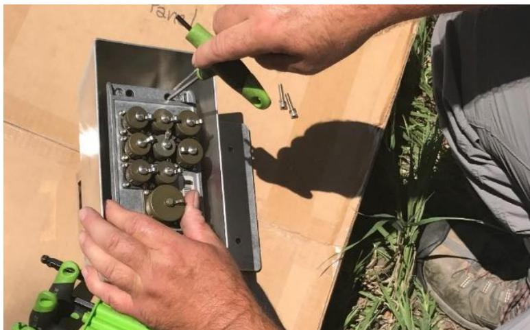
**Figure 46. Remove Grape from Grape Shields (D06 KING)**
