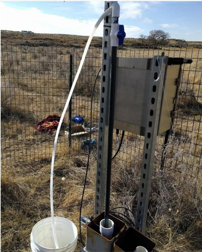
Figure 33. Set up Surge Block (D10 ARIK)
