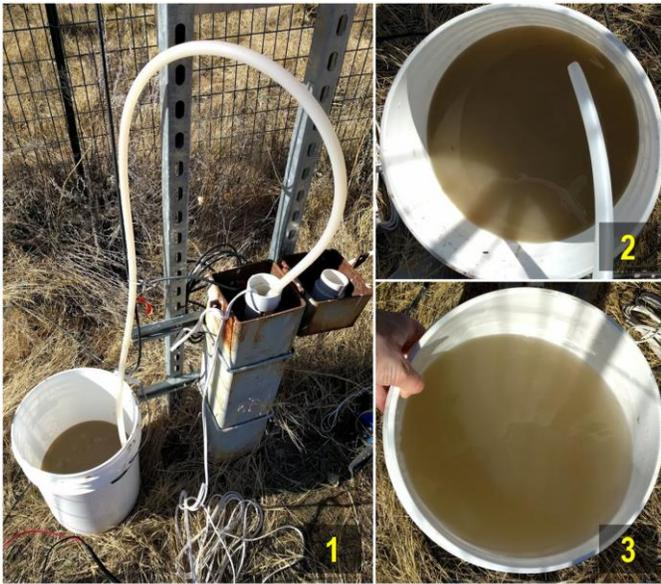
Figure 30. GWW Prep with Mini-Typhoon (D10 ARIK)
