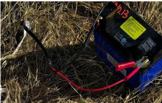
Figure 29. Connect Mini-Typhoon/Monsoon to 12V Battery (D10 ARIK)
