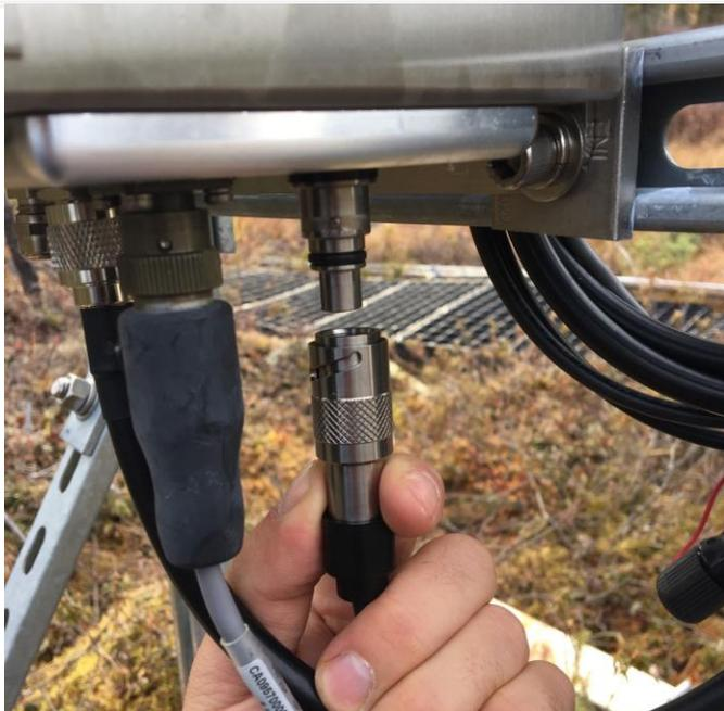
**Figure 48. Disconnect Sensor Cable (D19 CARI)**
