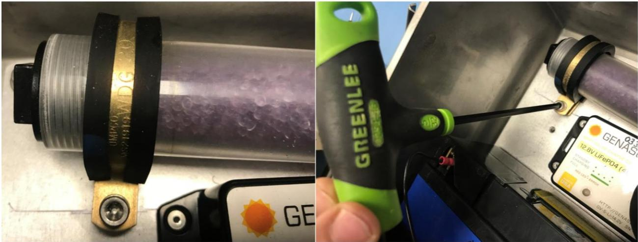
**Figure 22. Loosen Clamp Securing Desiccant Canister to Radio/Power Box Back Plate with 5/32 Hex Wrench**
