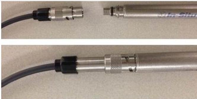
**Figure 57. Cable to Sensor Connectors**
