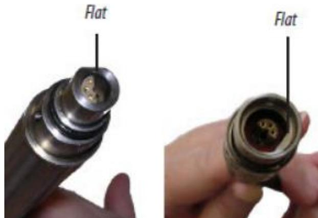
Figure 15. Aqua TROLL Connector "Flat" Side to Align Connectors
