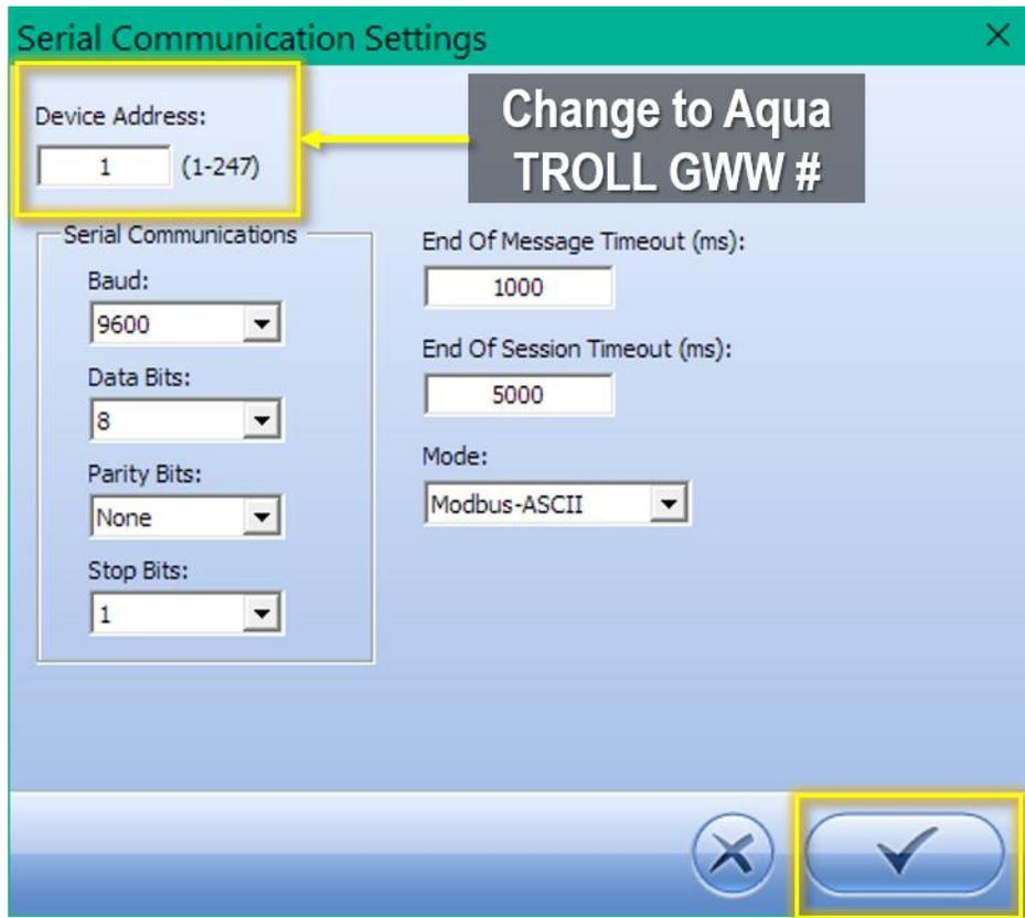
Figure 93. Update Device Number to Reflect Sensor GWW #
