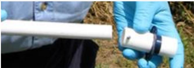
Figure 31. Assemble Surge Block (Source: ER [07])
