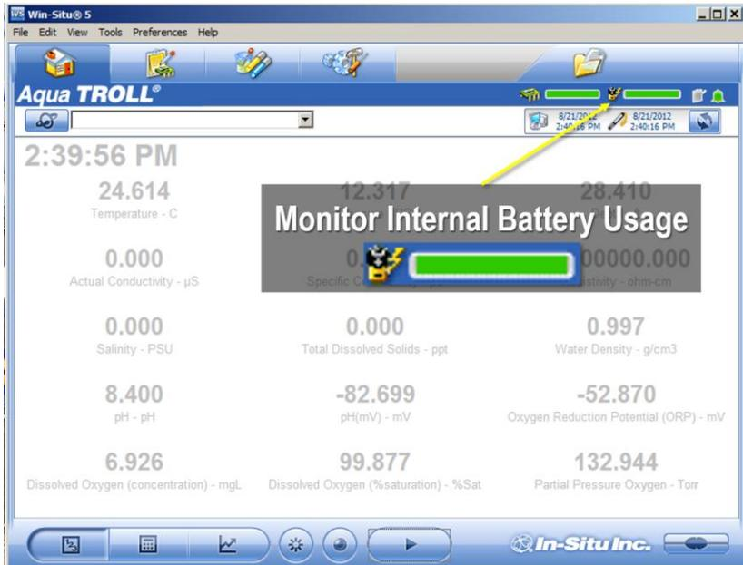
**Figure 44. Win-Situ 5 Internal Battery Status Bar Screenshot**
