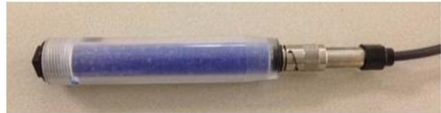
**Figure 58. Desiccant Canister to Vented Cable Connectors**
