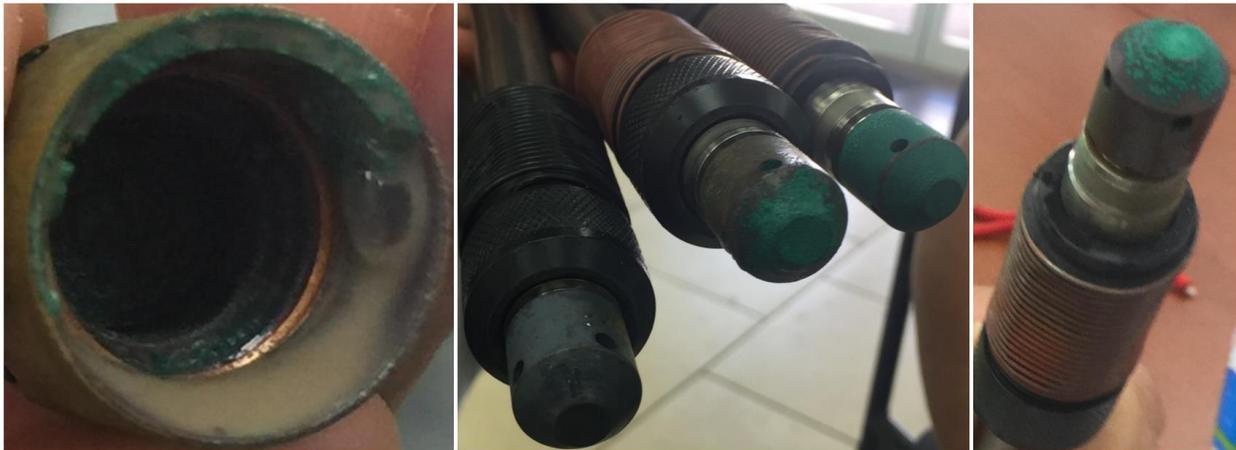
**Figure 11. Examples of Biofouling on Aqua TROLL 200**
