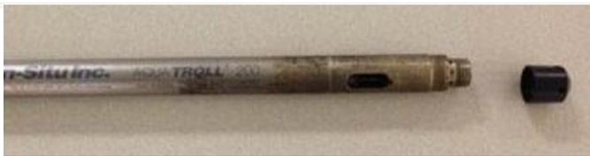
**Figure 54. Unthread Black Nose Cone from Sensor**
