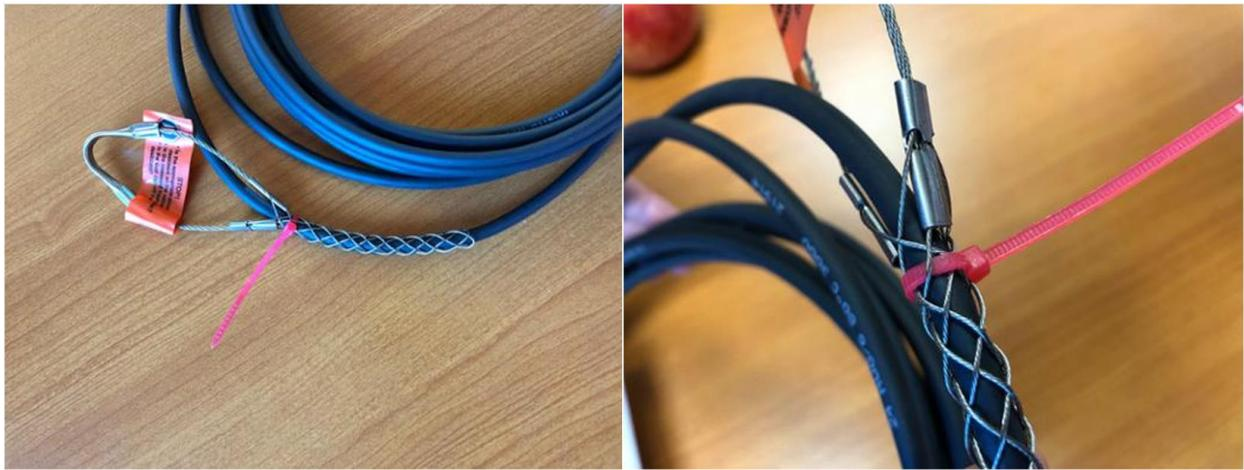
**Figure 19. Secure Mesh Wire Basket to Sensor Cable**
