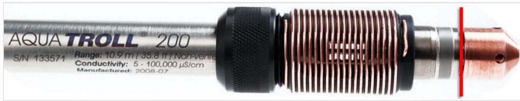
Figure 68. Red Line Identifies the Position to Measure for Sensor Cable Length
