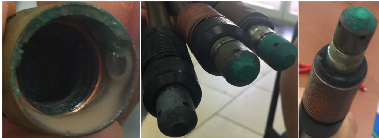
Figure 17. Examples of Biofouling on Aqua TROLL 200
