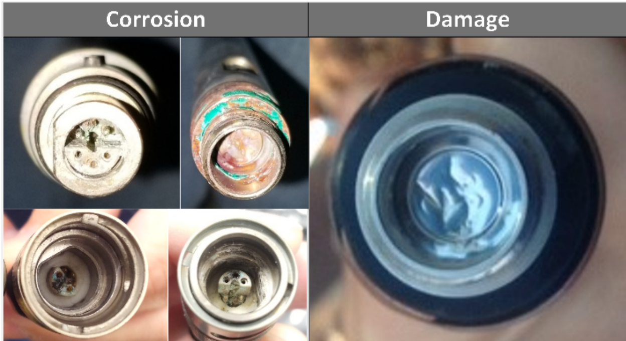
Figure 12. Examples of corrosion and damage on Aqua Troll 200 sensors.
