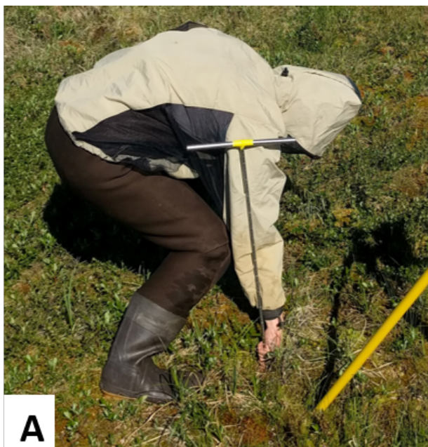
Figure 108. Measure thaw depth by inserting the thaw probe to the frozen interface (A) and reading the corresponding centimeter mark (B).
