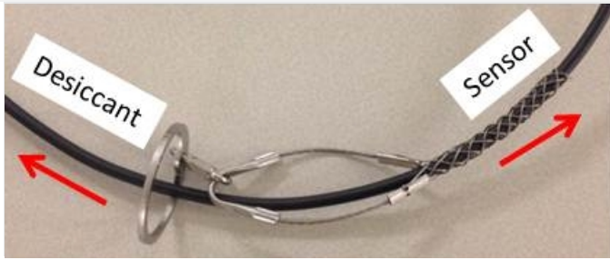
Figure 65. Cable and Wire Basket with Well Dock Orientation
