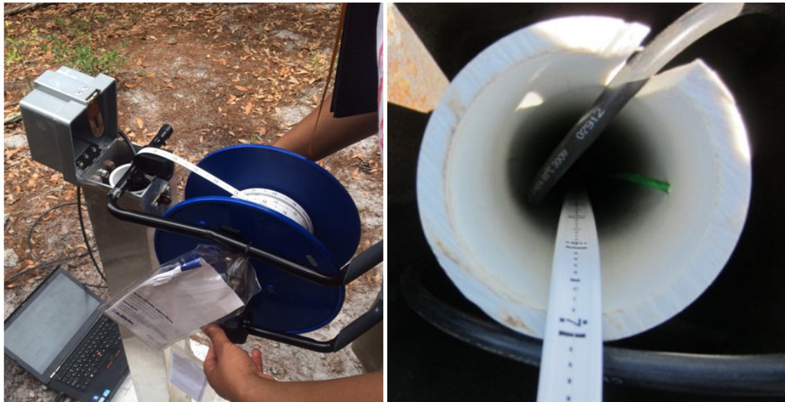
Figure 70. Water Level Tape to Measure Depth to Water
