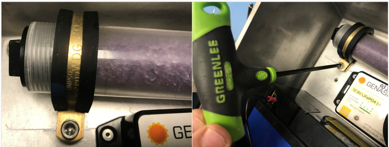
Figure 28. Loosen Clamp Securing Desiccant Canister to Radio/Power Box Back Plate with 5/32 Hex Wrench
