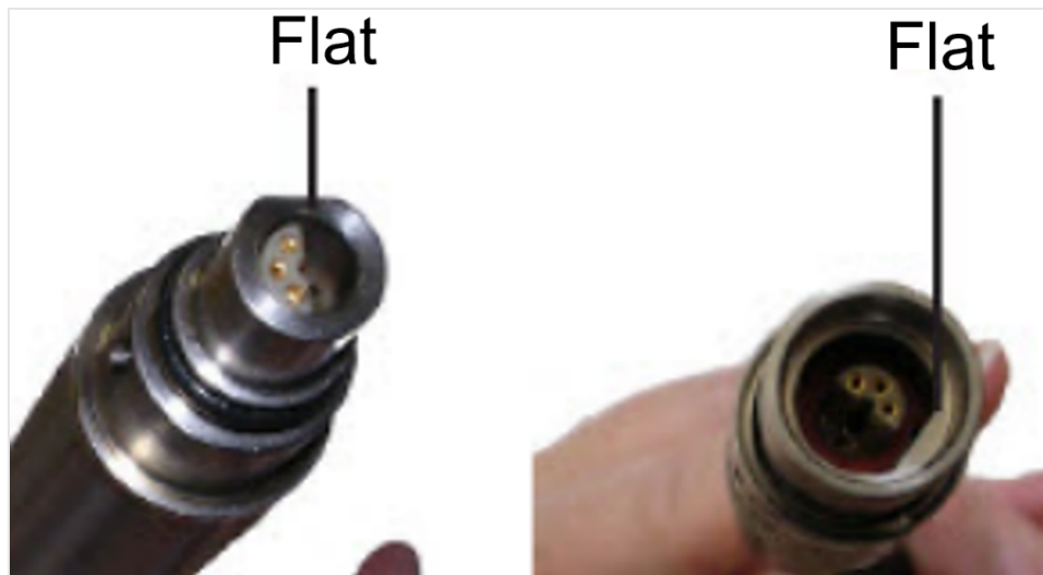
Figure 21. Aqua TROLL Connector "Flat" Side to Align Connectors
