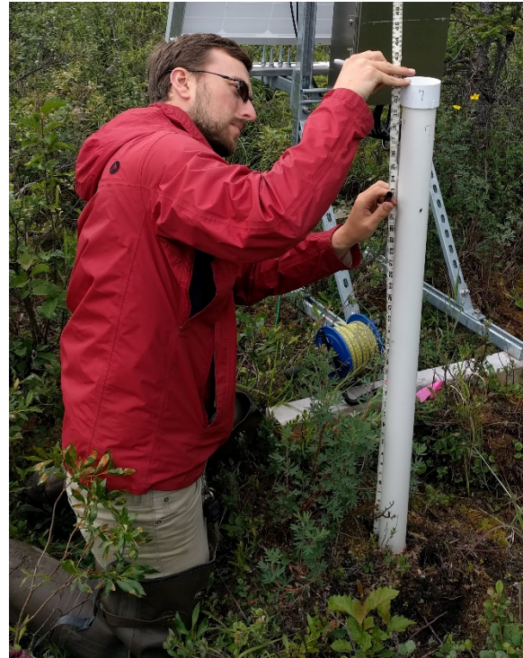
Figure 107. Measure from the Top of the GWW (with the cap removed) to the Ground Surface
