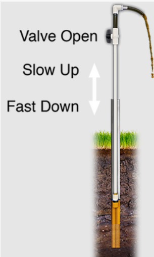
Figure 40. Flush GWW with Surge Block (ER [07])
