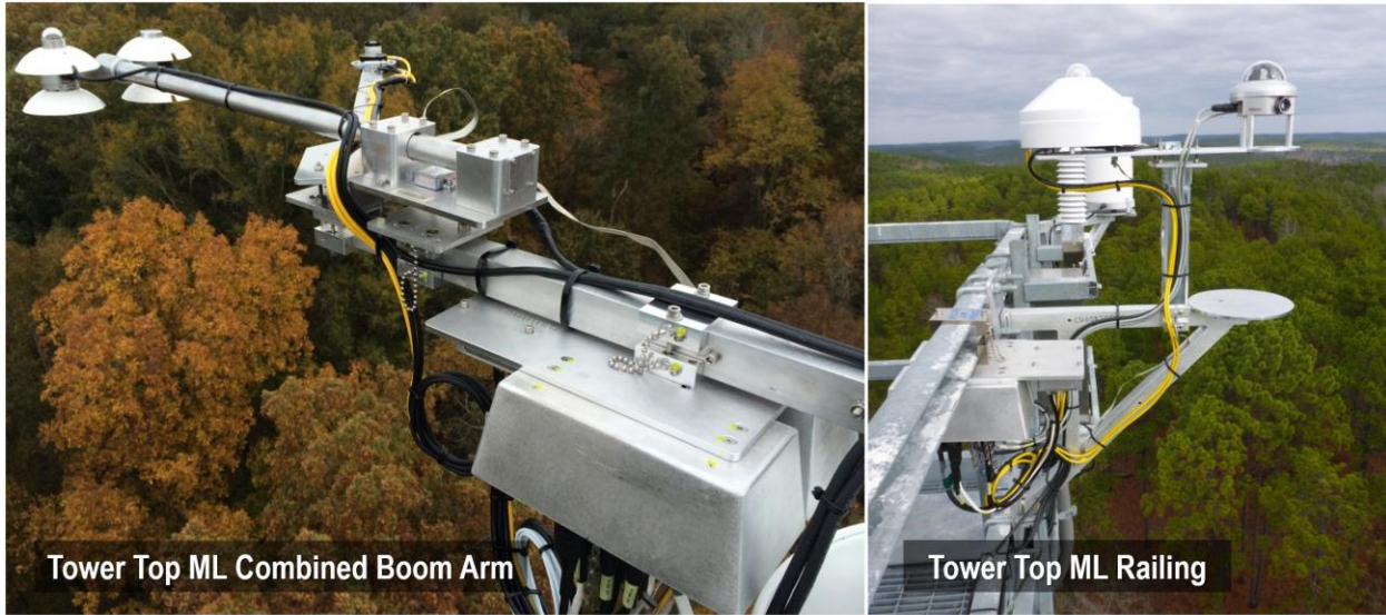
Figure 55. Tower Top ML Combined Boom Arm with Net Radiometer & PAR Quantum Sensor (D08 DELA) and Railing with the Primary Pyranometer and Sunshine Pyranometer (D08 TALL)
