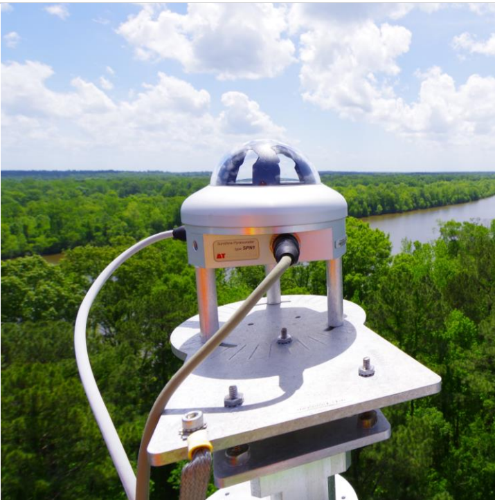
Figure 21. Sunshine Pyranometer mounted atop a TIS Tower.
