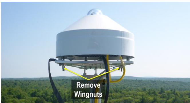
Figure 58. Remove the Primary Pyranometer from Mount Plate
