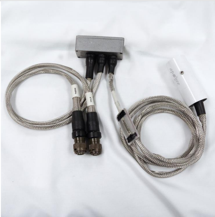
Figure 29. Biological Temperature Sensor and associated stainless steel braided cabling and connectors.
