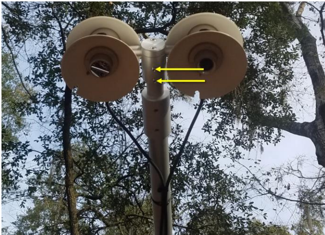
Figure 83. Remove Set Screws to Remove Net Radiometer
