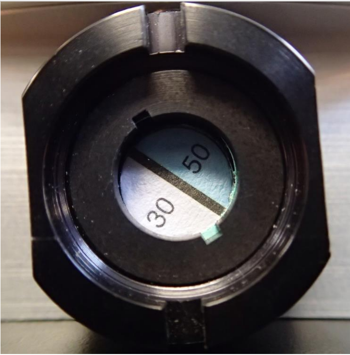
Figure 20. Close up of the Humidity Indicator Window on the Desiccant Canister. The numbers indicate 30% and 50% relative humidity (RH).
