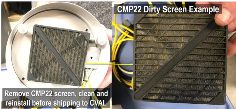
Figure 108. Primary Pyranometer Screen Requires Cleaning
