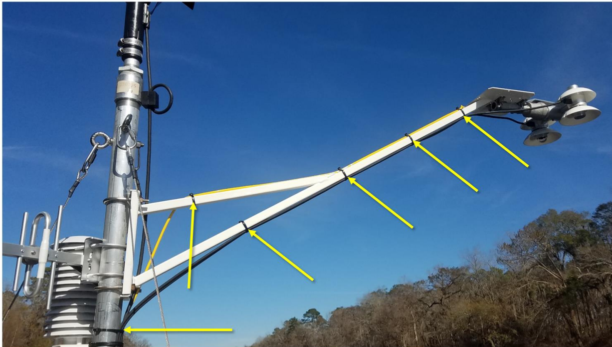
Figure 105. Re-dress Sensor Cables with Zip Ties (D03 FLNT)
