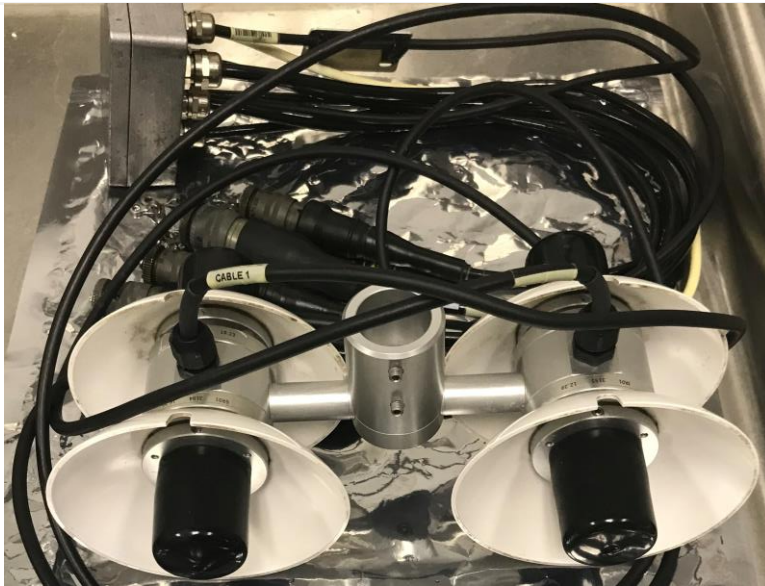
Figure 116. Net Radiometer with Black Caps over the sensors.
