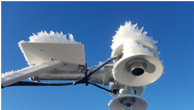
Figure 100. Radiation Sensor Winterization (D18 TOOL)
