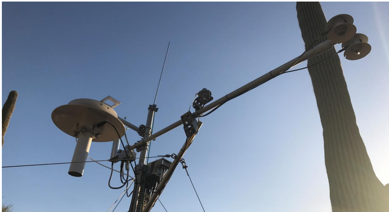
Figure 79. AIS Aquatic Met Station Radiation Boom Arm with PAR Quantum Sensor and Net Radiometer (D14 SYCA)
