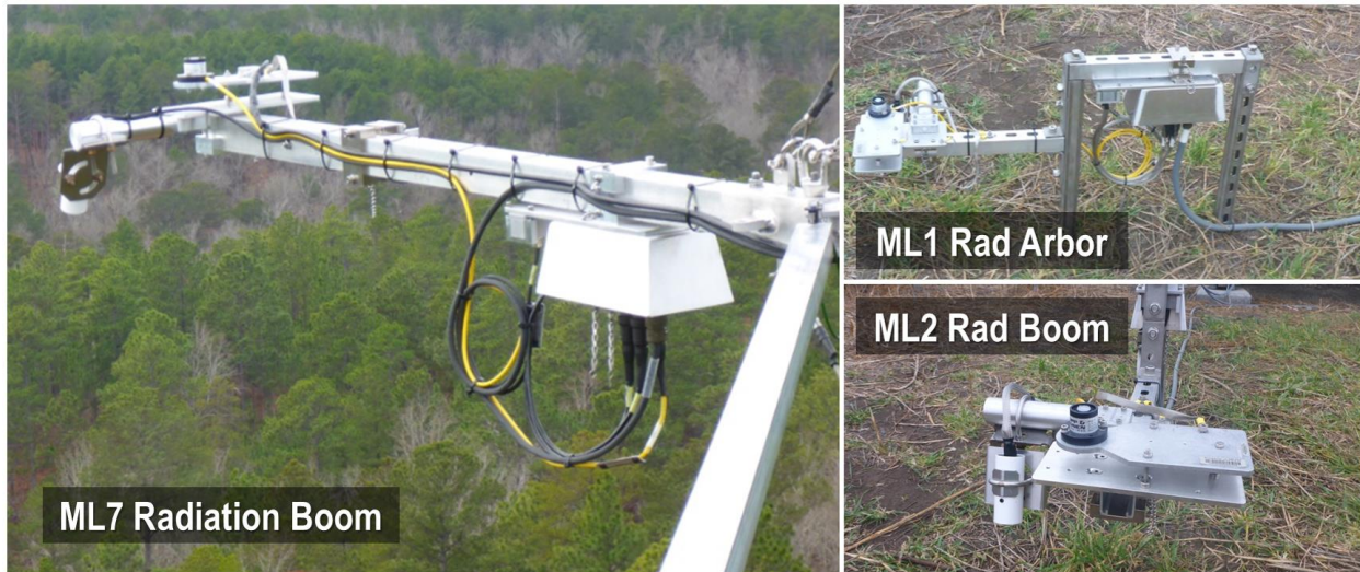
Figure 43. Tower Profile ML Radiation Booms/Arbor: Biological Temperature Sensor (SI-111) and PAR Quantum Sensor (PQS1)
