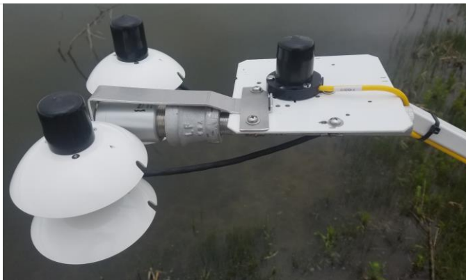
Figure 104. AIS Buoy Radiation Boom Arm: Net Radiometer and PAR Quantum Sensor with Black Caps over the Sensor Diffusers
