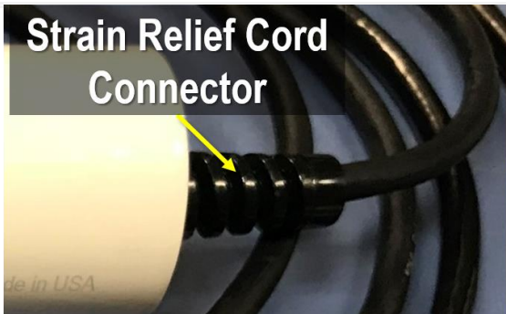
Figure 113. Biological Temperature Sensor Requires Cable Strain Relief – Use Zip Ties to Prevent Straining the Cable if the Sensor has No Connector
