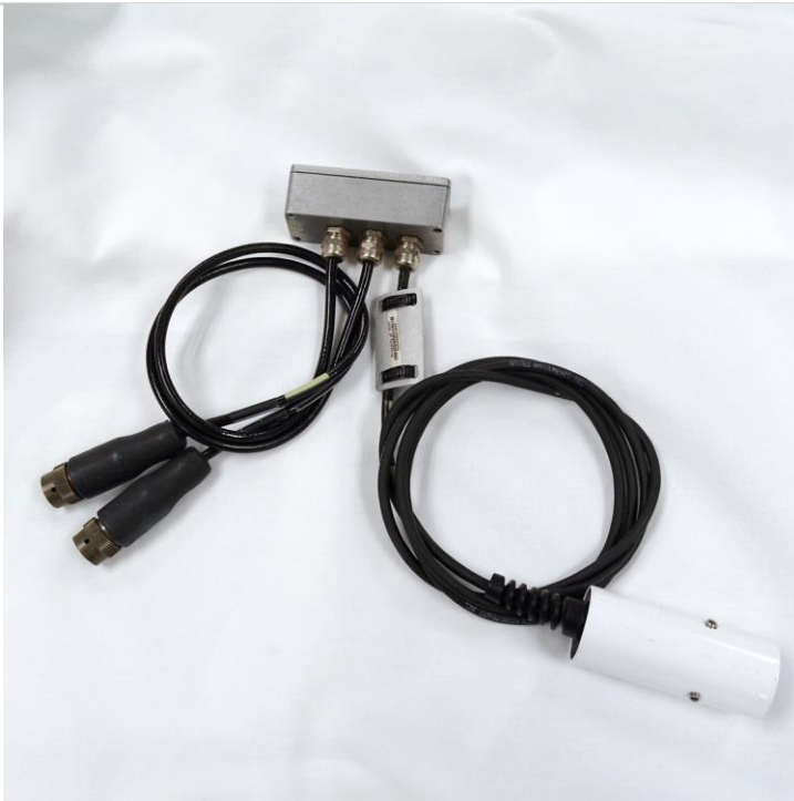
Figure 28. Biological Temperature Sensor and associated TPE jacketed cabling and connectors.
