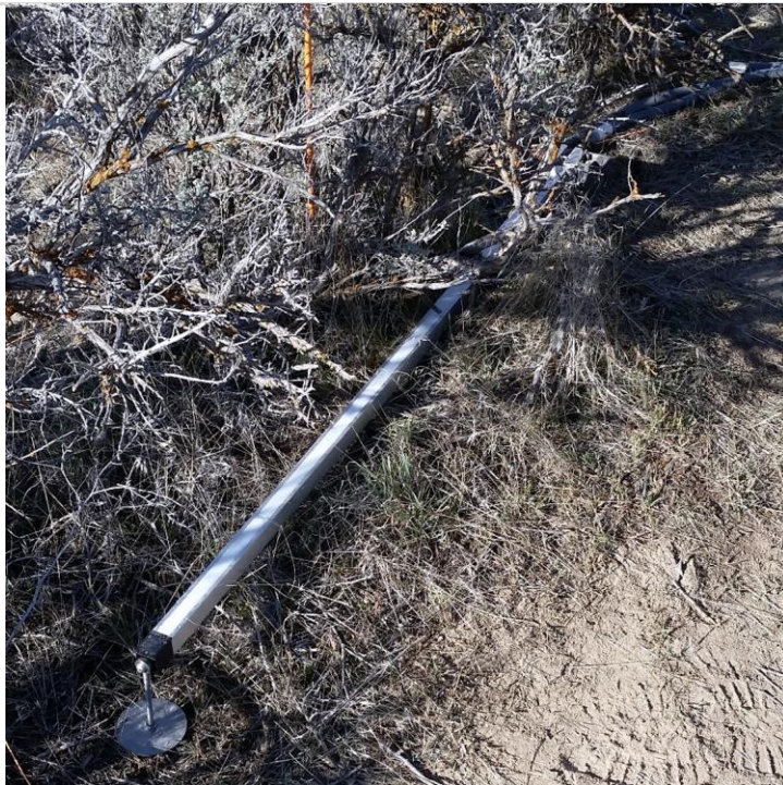
Figure 40. Quantum Line Sensor installed underneath some vegetation within a soil plot.
