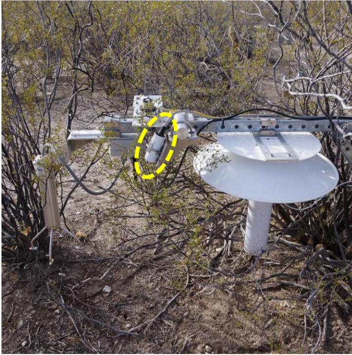
Figure 31. Biological Temperature Sensor mounted on ML1 along with other sensors.
