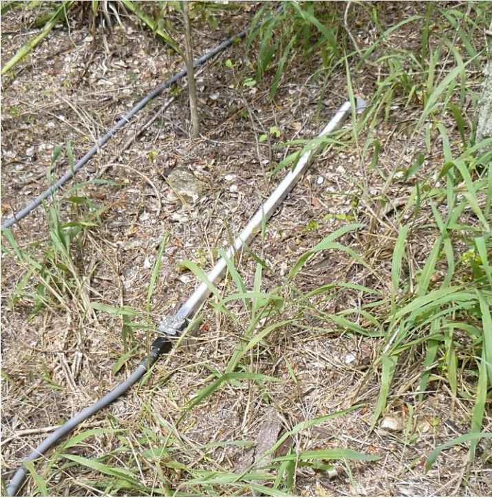
Figure 41. Quantum Line Sensor installed within a soil plot.
