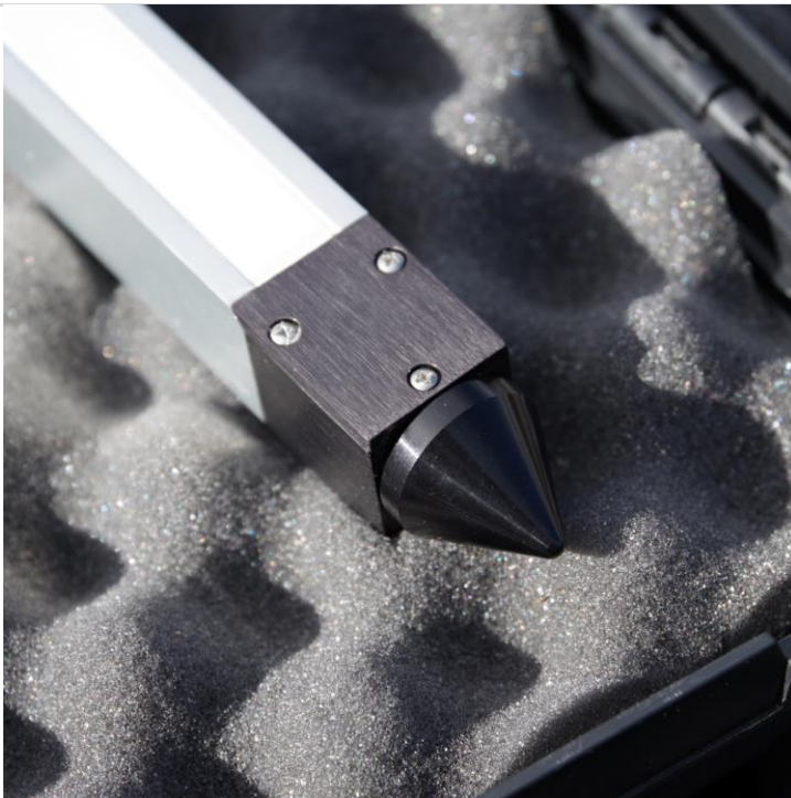
Figure 38. Close-up of the "cone" end of the Quantum Line Sensor.
