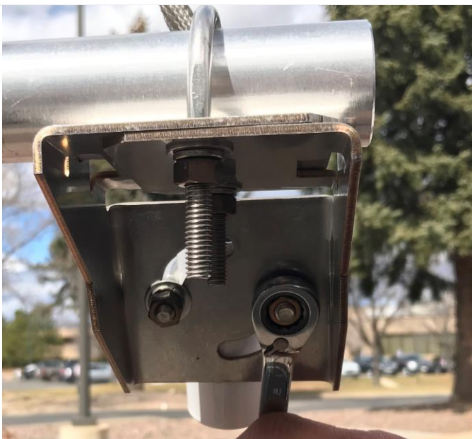
Figure 46. Remove PAR Quantum Sensor with 5/32" Allen Wrench
