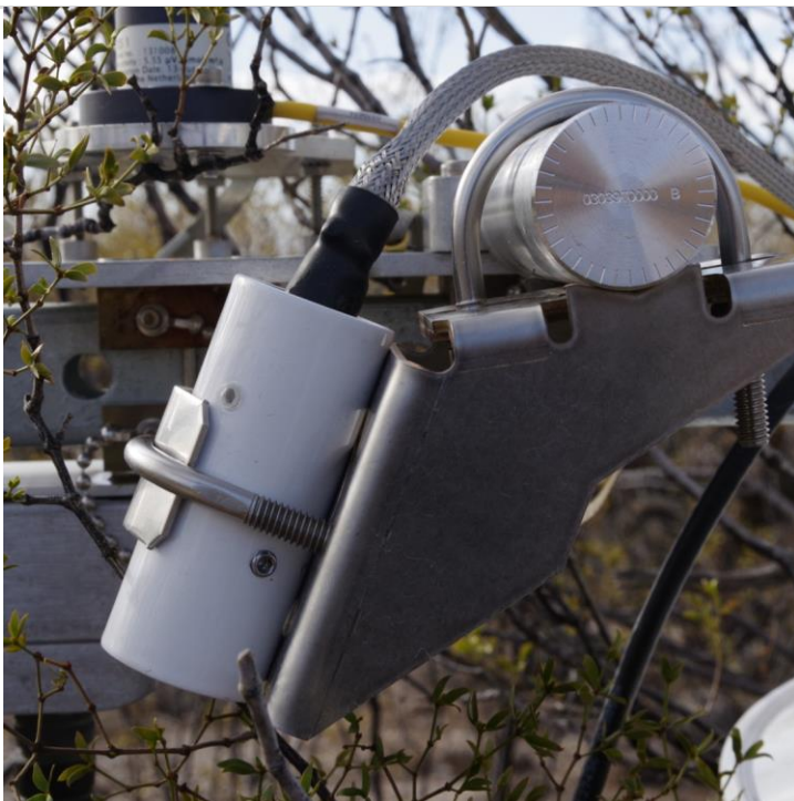
Figure 30. Biological Temperature Sensor mounted 22° from vertical.
