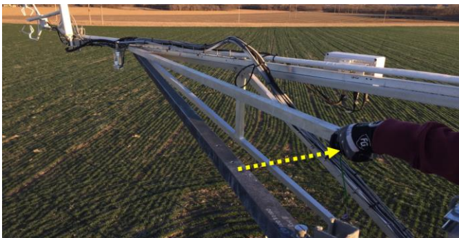
Figure 65. Guide the Boom Arm Toward the Tower Top (D06 KONA)
