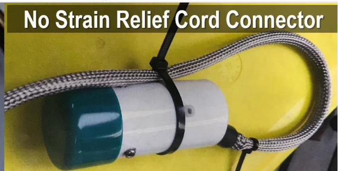
Figure 113. Biological Temperature Sensor Requires Cable Strain Relief – Use Zip Ties to Prevent Straining the Cable if the Sensor has No Connector
