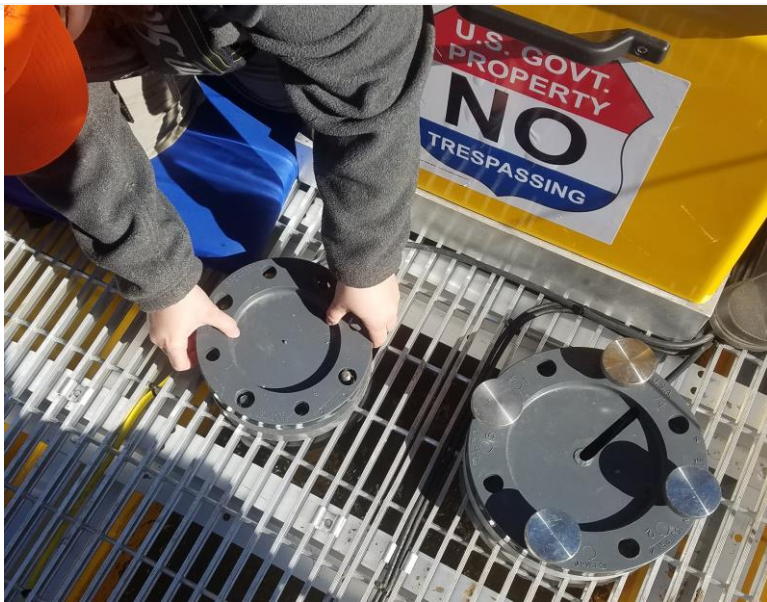
Figure 77. Lift Cap to Access Sensor in Tube
