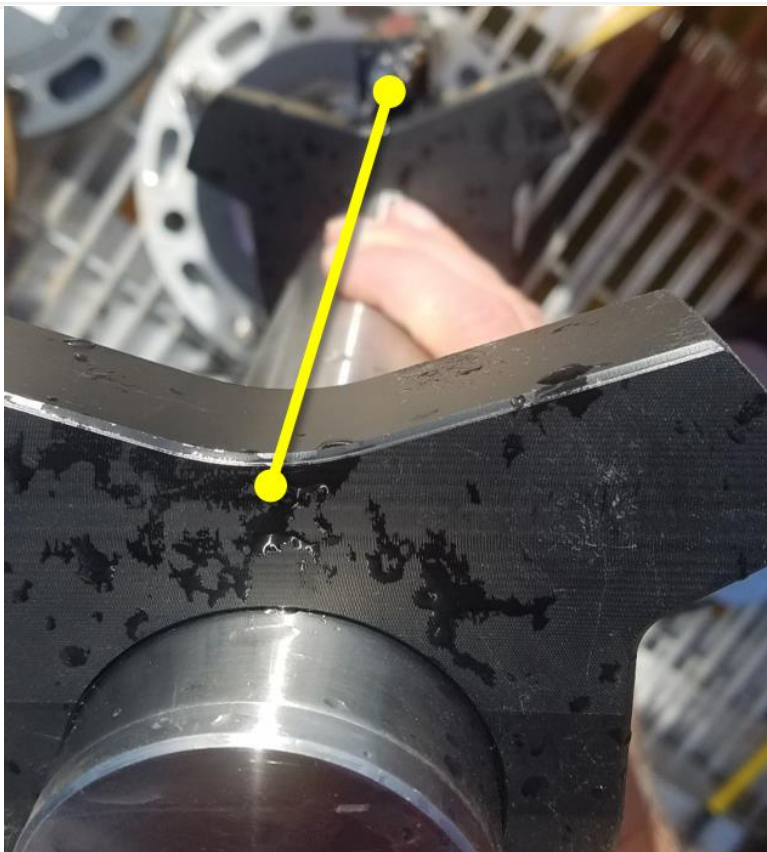
Figure 82. SUNA Wiper Placement
