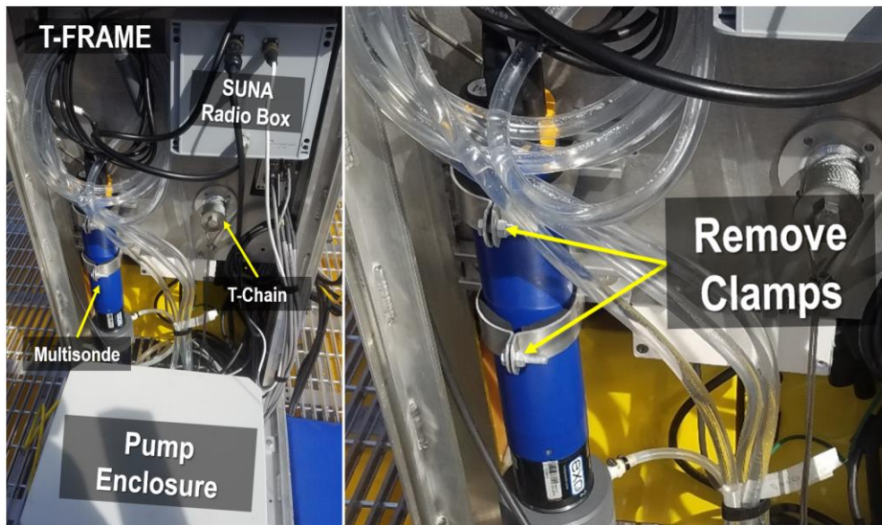
Figure 55. Use Wrench to Remove the Multisonde from the Two Clamps
