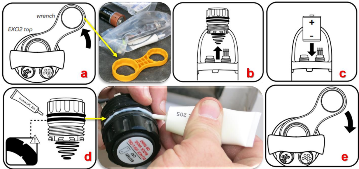
Figure 51. How to Replace Multisonde Internal D-Cell Batteries and Grease O-Rings (Source: ER [16] )
