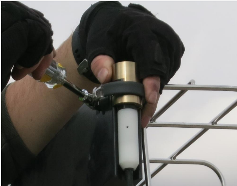
Figure 63. Use Screwdriver or Nut Driver to Remove uPAR Sensor from Mount
