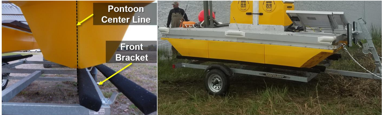
Figure 29. Mounting the AIS Buoy on the Trailer
