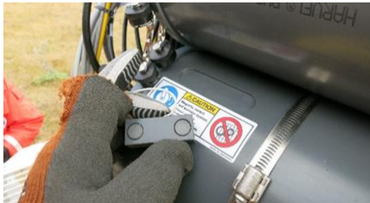
Figure 49. Magnetic Switch to Activate the Winch
