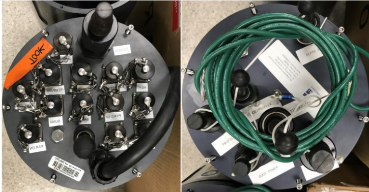
Figure 101. MET Canister and Profiler Canister (NOTE: DISREGARD GREEN GROUND WIRE – KEEP GROUND WIRE AT DOMAIN)
