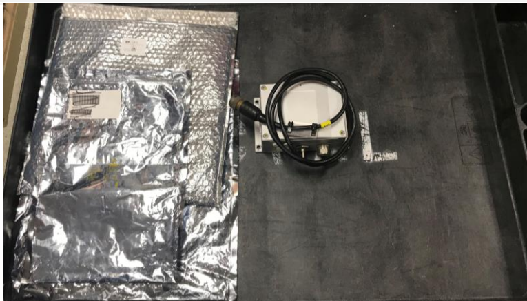
Figure 95. Vaisala Barometric Pressure Sensor - Requires ESD Packaging
