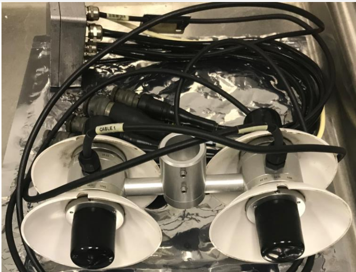
Figure 98. NR01 with Black Caps over Diffuser – Req. ESD
