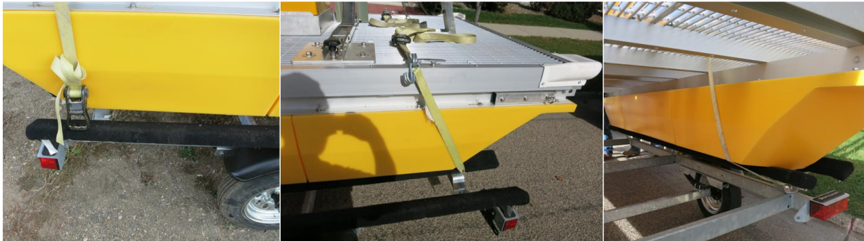
Figure 44. Ratchet Straps secure the AIS Buoy to the Trailer
