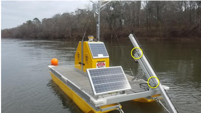
Figure 70. Release Two Slide Locks to Bring Extension Bar uPAR Mount Above Water
