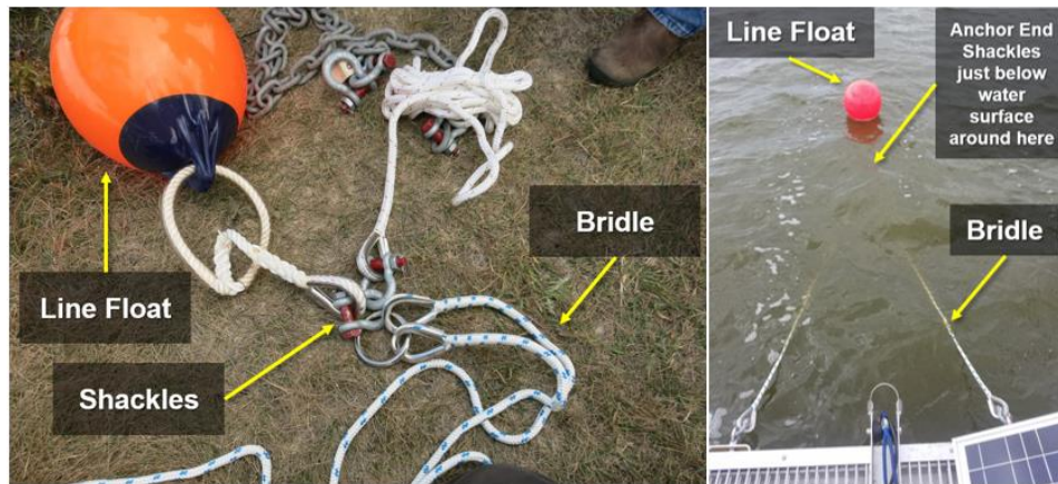
Figure 11. Shackles at the Anchor End of Bridle with Line Floats
