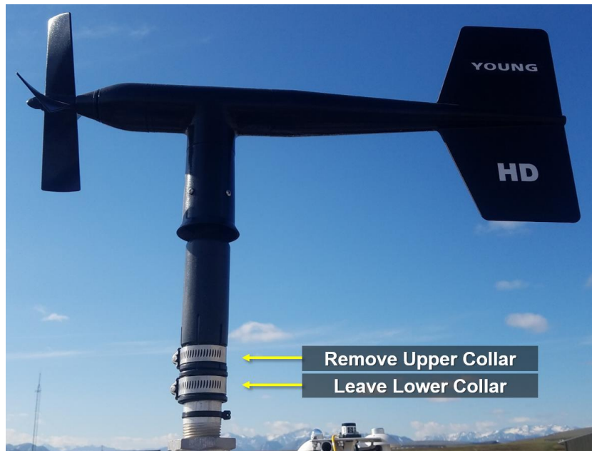
Figure 41. RM Young Wind Monitor (2D Wind) Upper and Lower Collar on Met Mast
