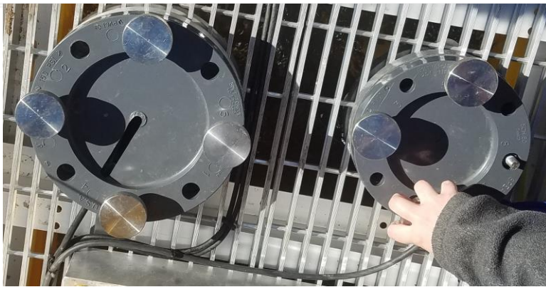
Figure 80. Align Cable with Notch where Cap/Lid mates with bottom Flange
