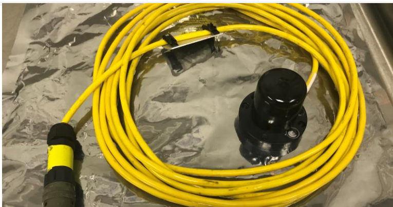
Figure 96. PQS1/PAR Sensor with Black Cap over Diffuser – Req. ESD
