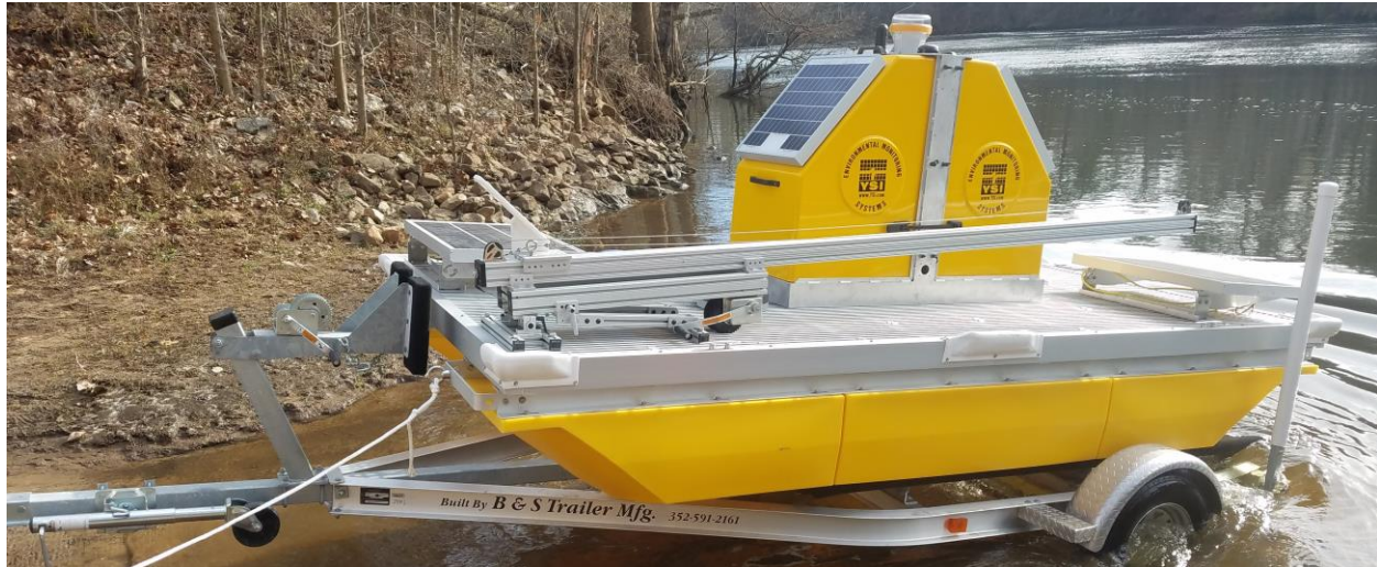
Figure 34. D03 FLNT ONLY: Retractable PAR Mounting System Flat on Deck for Transport
