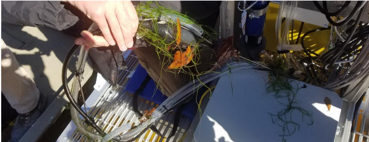
Figure 28. D03 FLNT: Pump Tubing pulled from the River
