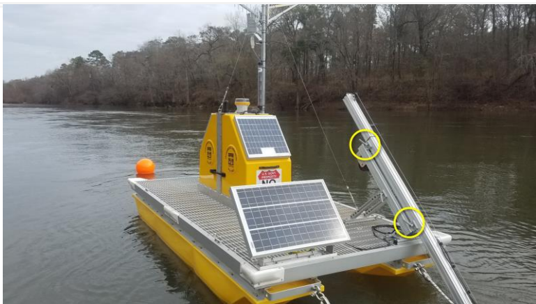
Figure 72. Lock Slide Locks to Secure Sensors Above Water
