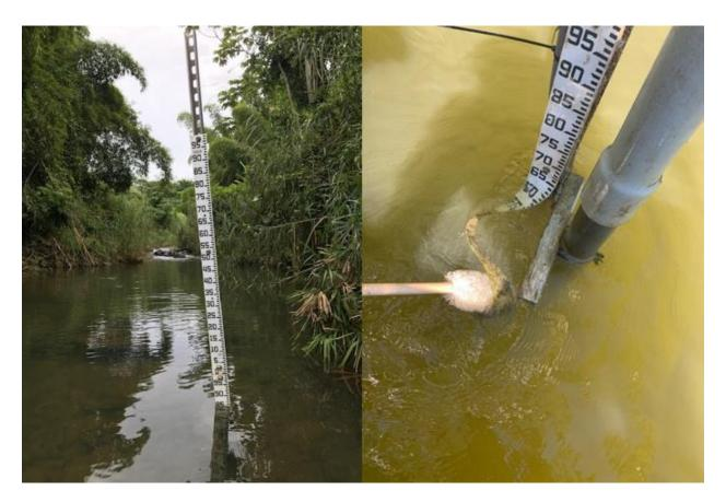
Figure 2. Examples of gauges needing repair.
