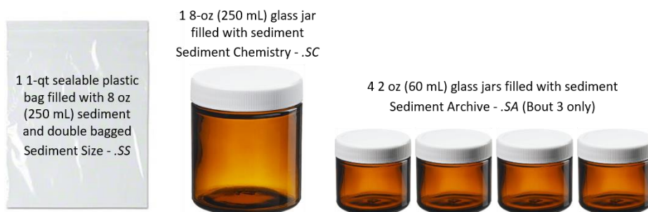
Figure 6. Example of amber glass jars with PTFE lined lid used for collecting sediment chemistry analyses and the sediment archive. Sediment for size analyses are collected in a 1 qt plastic sealable bag filled with approximately 8-16 oz (250-500 mL) of sediment and double bagged.
