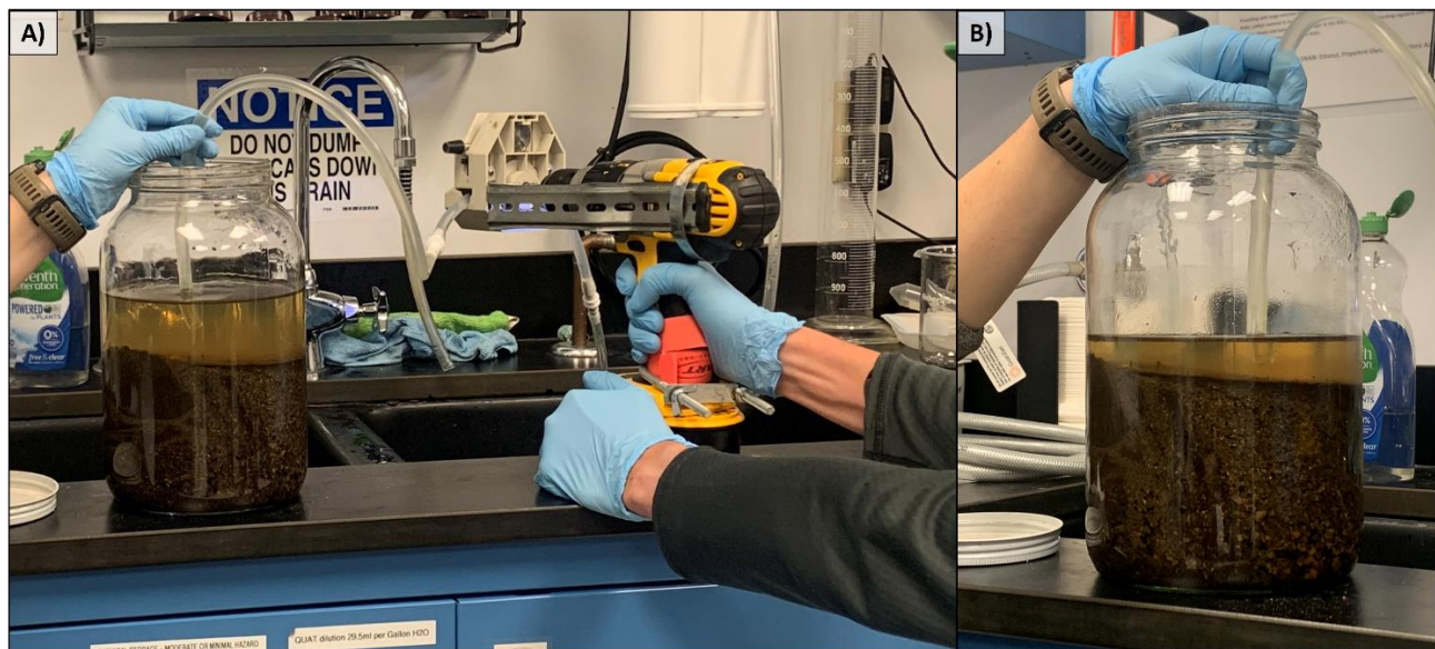
Figure 22. Decanting from the composite sample jar into a sink using the peristaltic pump.
