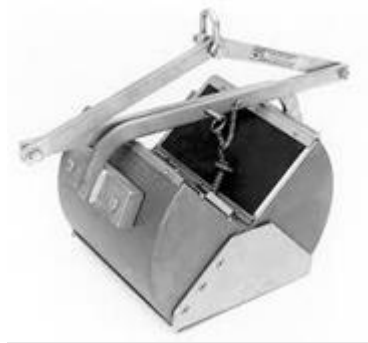
Figure 20. Petite Ponar® sampler for use in lakes and non-wadeable streams.
