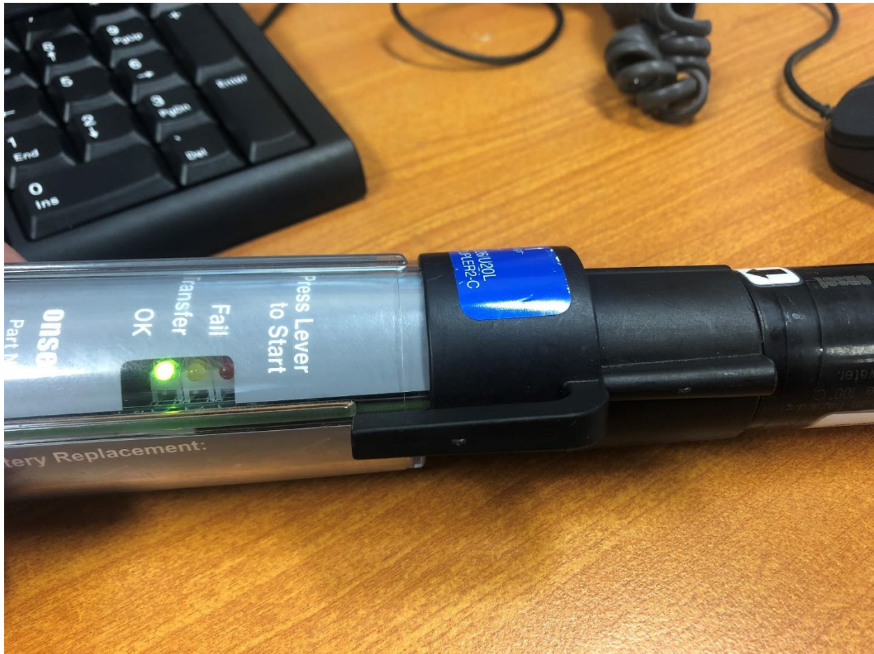
Figure 6. A green light indicates a successful data transfer from the logger to the shuttle after pressing the lever to start the transfer.
