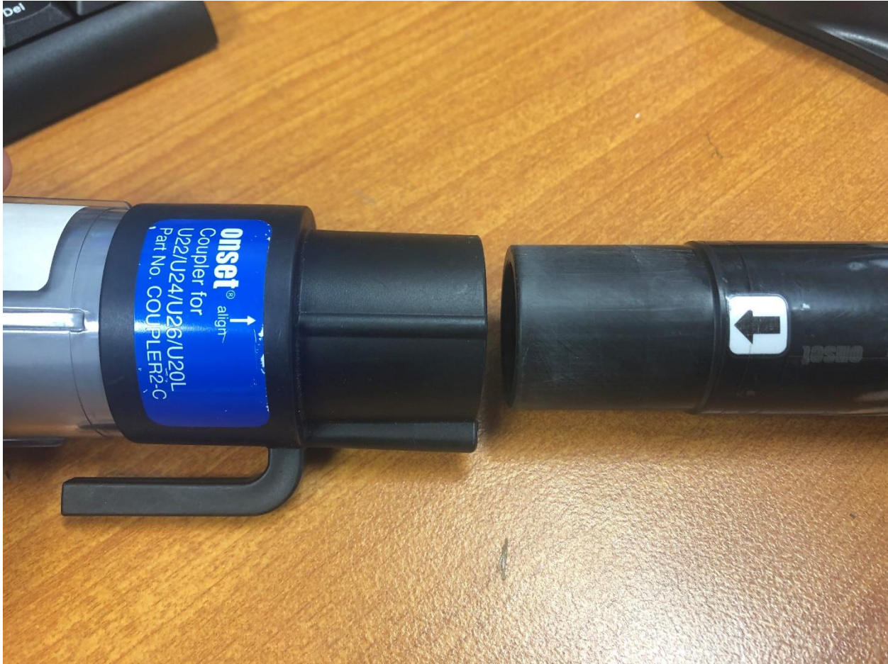
Figure 5. Plug a HOBO U24 logger into the shuttle with the coupler attached. Ensure proper alignment. This is ideally performed while the shuttle is connected to a laptop with HOBOWare Pro installed so that you can re-sync the logger's time in UTC (GMT).
