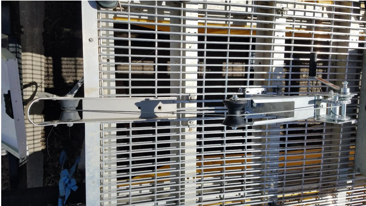
Figure 4. Top-down view of winch system with retrieval line routed through the winch assembly.
