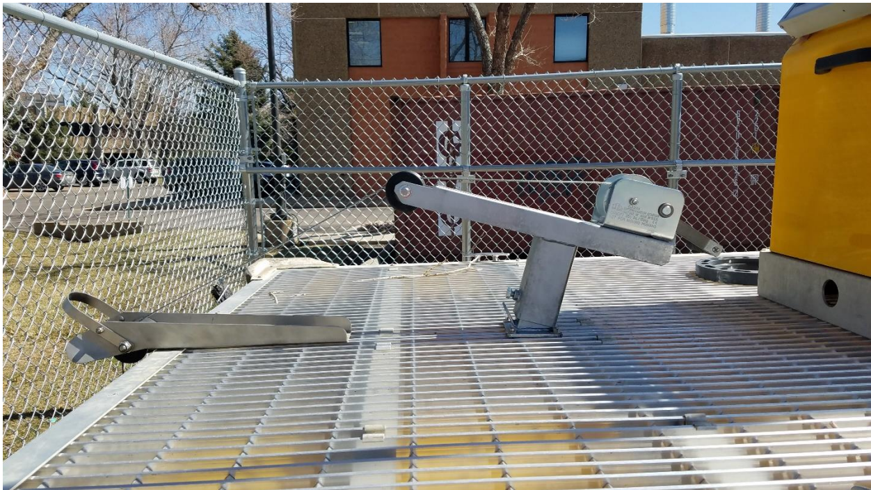
Figure 3. Side profile of winch system with bow roller with retrieval line routed through the bow roller and onto the hand crank winch.
