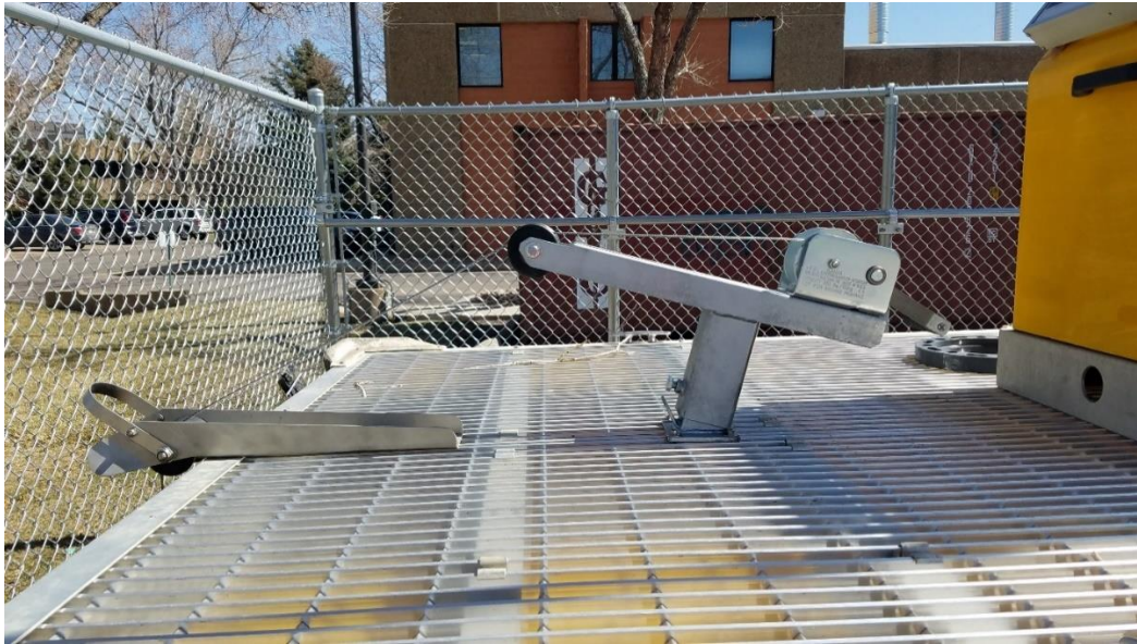
Figure 4. Side profile of winch system with bow roller with the retrieval line routed through the bow roller and onto the hand crank winch.
