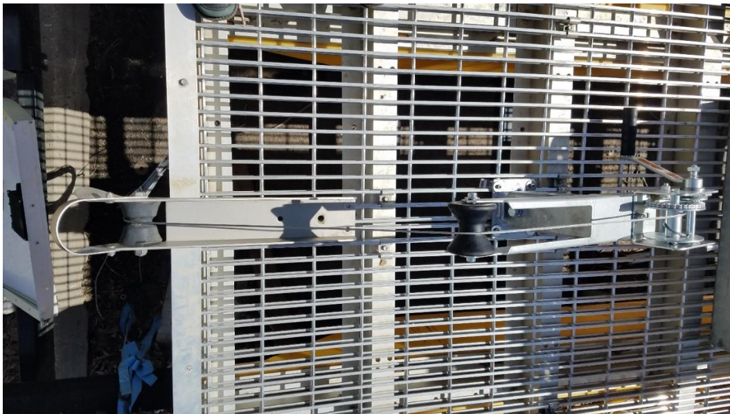
Figure 5. Top-down view of winch system with retrieval line routed through the winch assembly.
