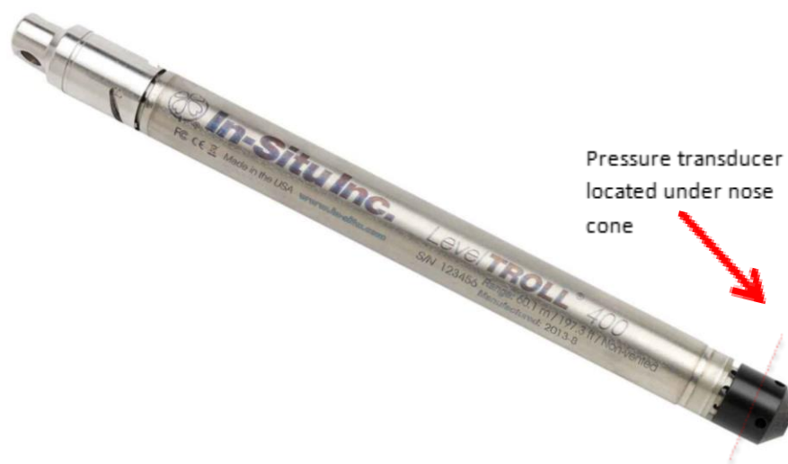
Figure 3. Photo of a Level Troll 500 with dashed red line indicating the location of the sensing mechanism under the nose cone.
