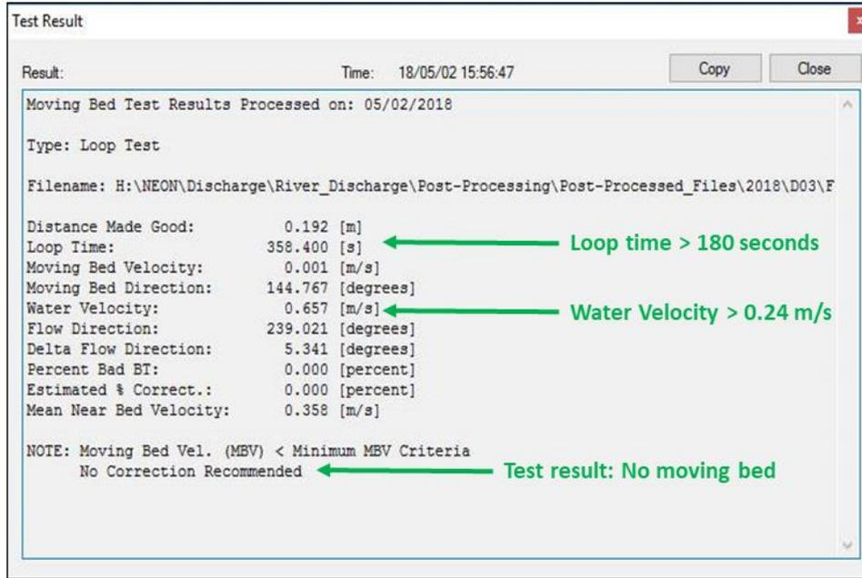
**Figure 8.** Moving Bed Loop Test Result window. In this example the required conditions were met to in order to evaluate whether a moving bed was present (Loop time, water velocity, and bottom tracking). A moving bed was not detected (the moving bed velocity < the moving bed velocity criteria) and no correction is recommended.
