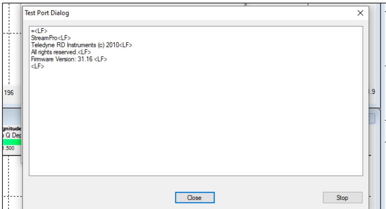
**Figure 3.** ADCP Test Port Dialog indicating that ADCP data are streaming from the ADCP to the laptop.
