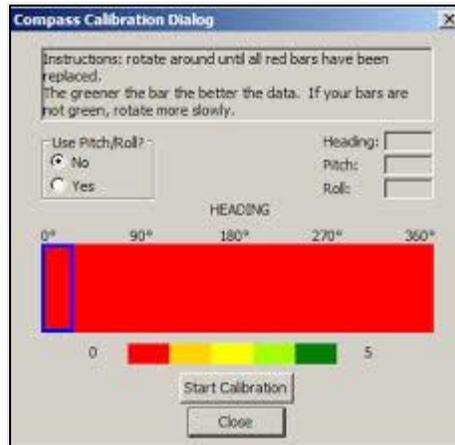
**Figure 6.** WinRiver II compass calibration dialog box. Upon initializing the compass calibration, all bars begin as bright red as shown above. Perform the compass calibration until all bars are the dark green color indicated in the far right side of the color scale.
