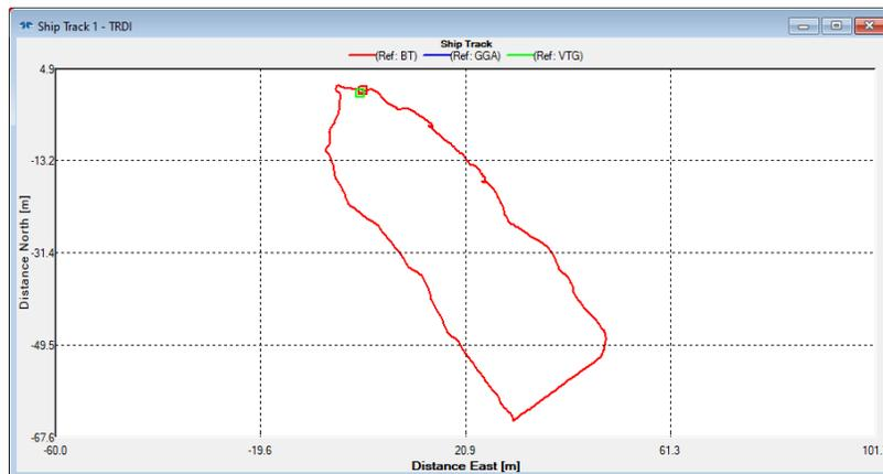
**Figure 7.** The WinRiver II Ship Track window displaying a Loop moving bed test. The green box indicates the ADCP starting position; the line shows the ADCP path as it navigates across the channel and turns back around toward the starting bank; the red box indicates the ADCP ending position. In this example, a moving bed is not present as the loop is closed and the red box is on top of the green box.
