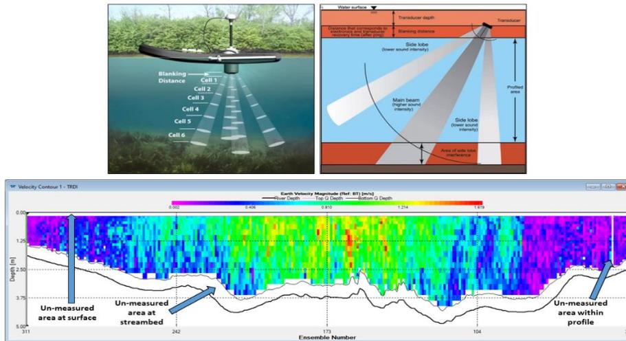
**Figure 11.** Unmeasured areas in the ADCP profile where velocity is extrapolated. Top left: ADCP blanking distance and cell size distribution; top right: unmeasured areas of the profile relative to ADCP beams (credit: SonTek); below: a velocity contour profile graph in WinRiver II with unmeasured areas delineated. Channel edges are not shown but constitute the third unmeasured area along with the top and bottom of the channel.
