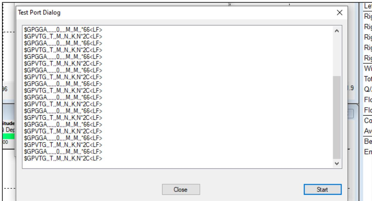
**Figure 4.** GPS Test Port Dialog indicating the Sirius XS Blue GPS data are streaming from the GPS antenna to the laptop.
