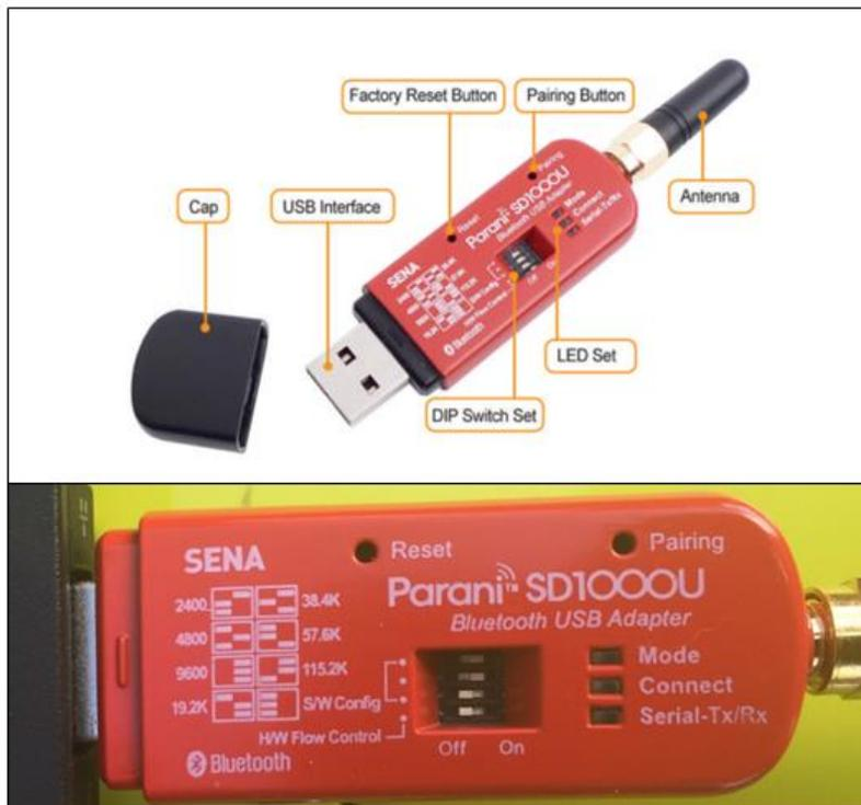
**Figure 2.** Top: Parani-SD1000U USB Bluetooth Adapter with default settings; Bottom: Correct settings for ADCP and GPS Bluetooth configuration.
