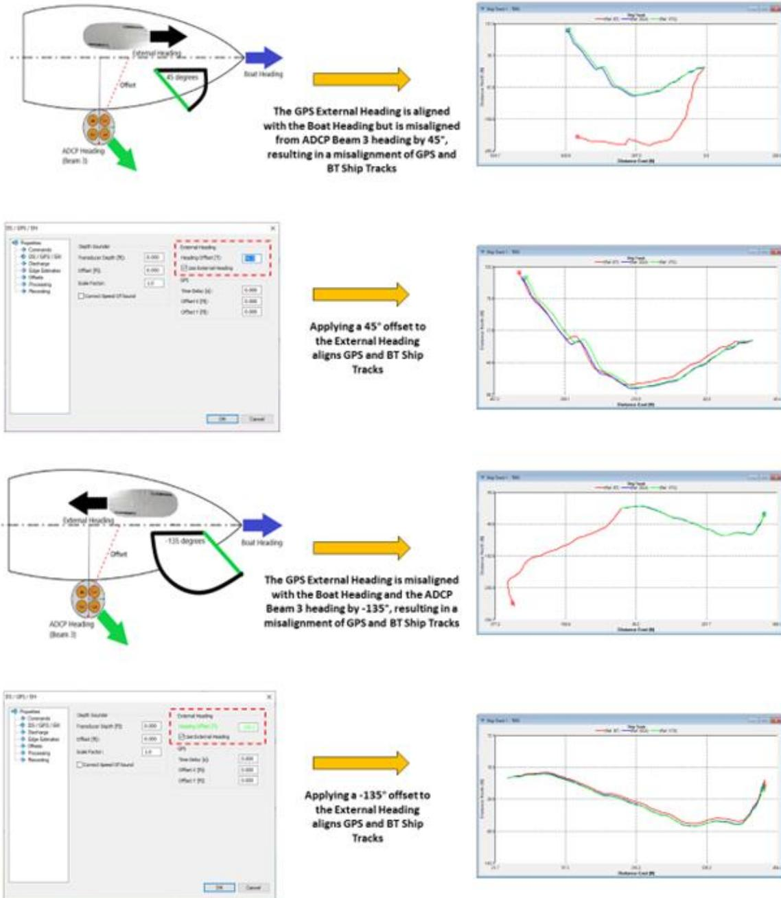
Figure 13. Applying External Heading offsets to align GPS and Bottom Track Ship Tracks.
