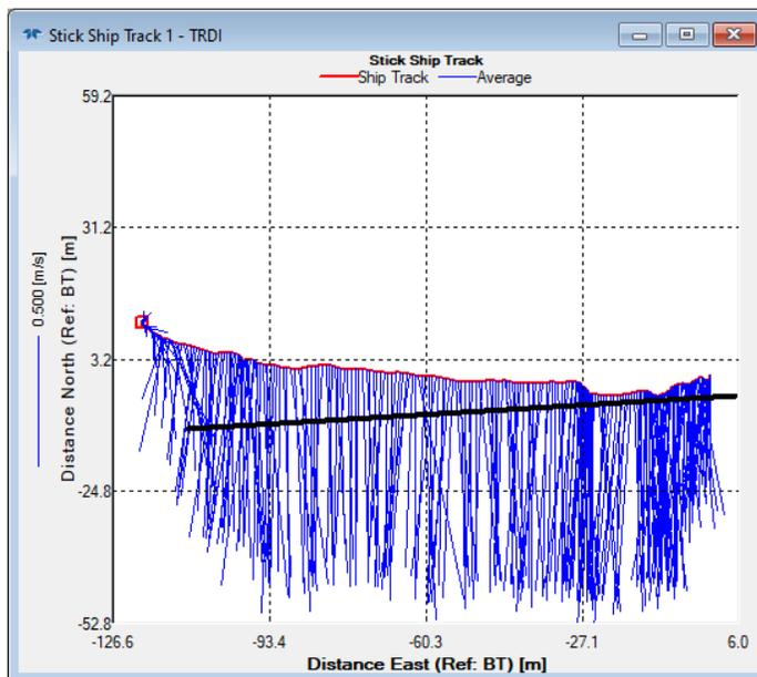
**Figure 15.** The Stick Ship Track window with the line of the transect (red) displayed alongside the line of the saved transect location (black) and velocity vectors (blue).
