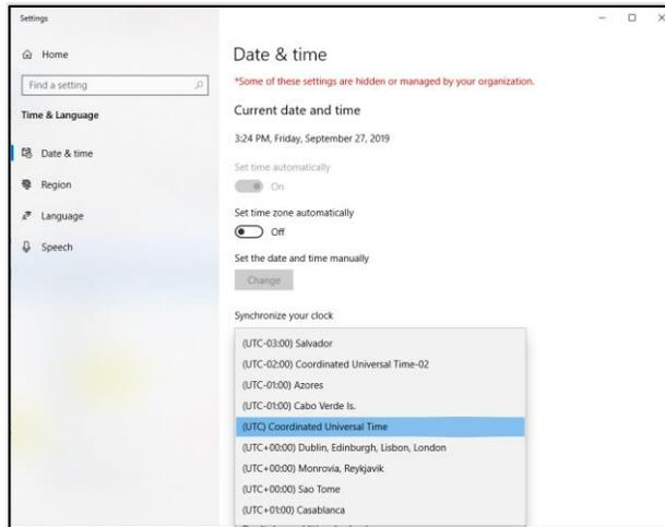
**Figure 5.** Set the PC used for the ADCP measurement to (UTC) Coordinated Universal Time and match the ADCP clock to this setting.
