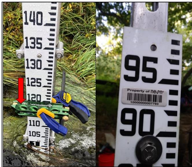
**Figure 11.** Left: NEON staff gauge where a clamp is placed to level the prism rod at the 1.20 meter mark, the red arrow indicates where the prism rod point is to be placed. Right: the staff gauge asset tag.
