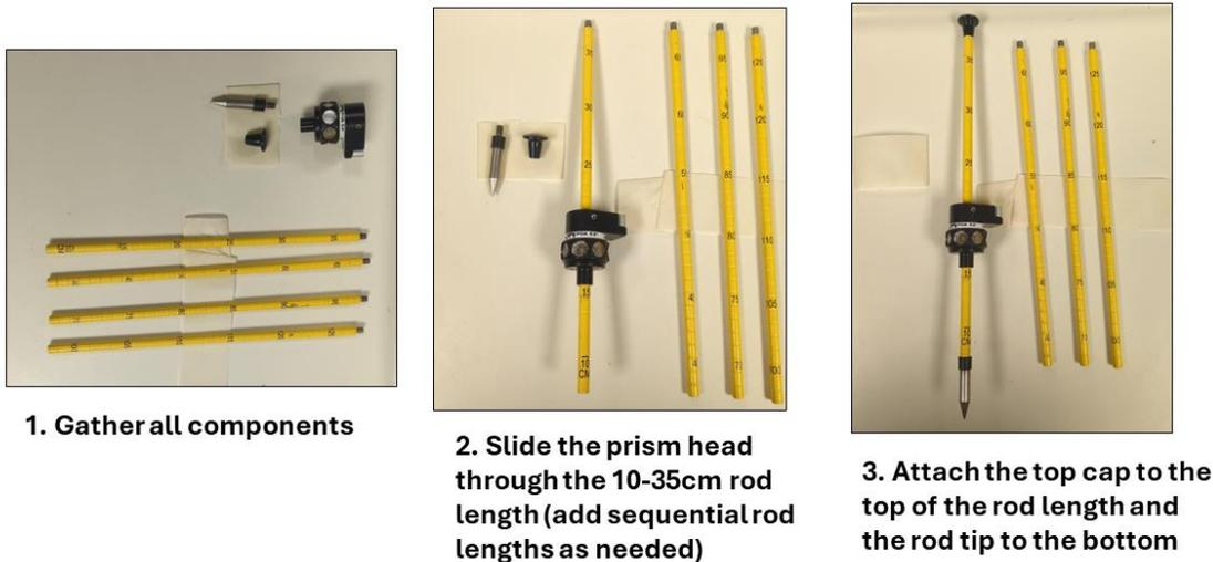
**Figure 16.** Steps to assemble the Sliding Mini Prism.
