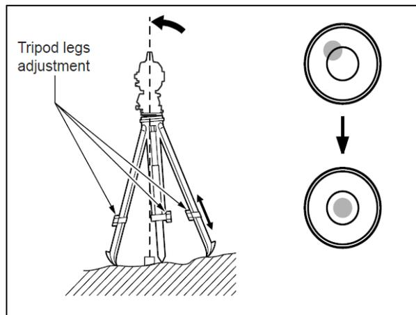
**Figure 5.** Leveling the tripod using the bubble level.
