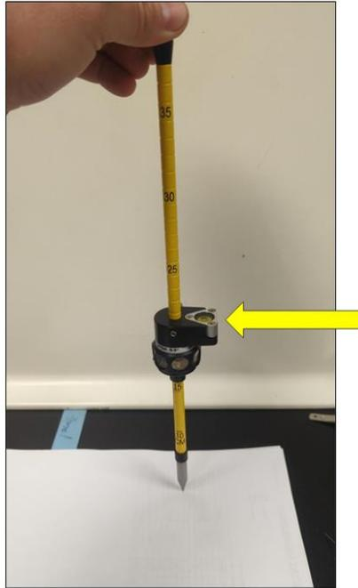
**Figure 19.** Arrow indicating the bubble level on the Sliding Mini Prism head.
