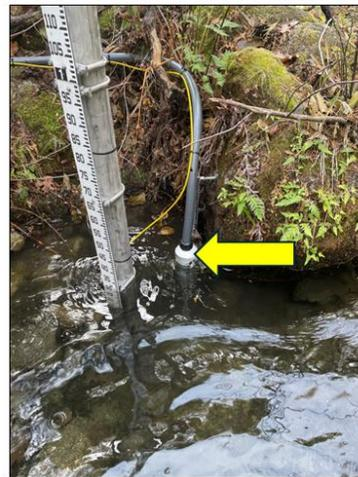
**Figure 13.** Left: Horizontally-installed Level TROLL with the yellow arrow indicating the divot where the point shall be mapped; Right: vertically-installed Level TROLL with the yellow arrow indicating the PVC cap, which is to be removed so that the point is mapped on the lip of the PVC
