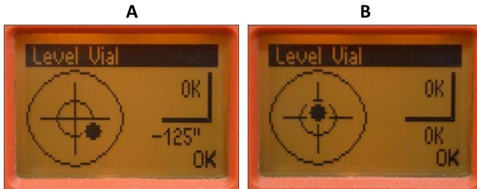
**Figure 6.** Total station fine-tuning leveling screen. A) The total station is not level; B) The total station is level.
