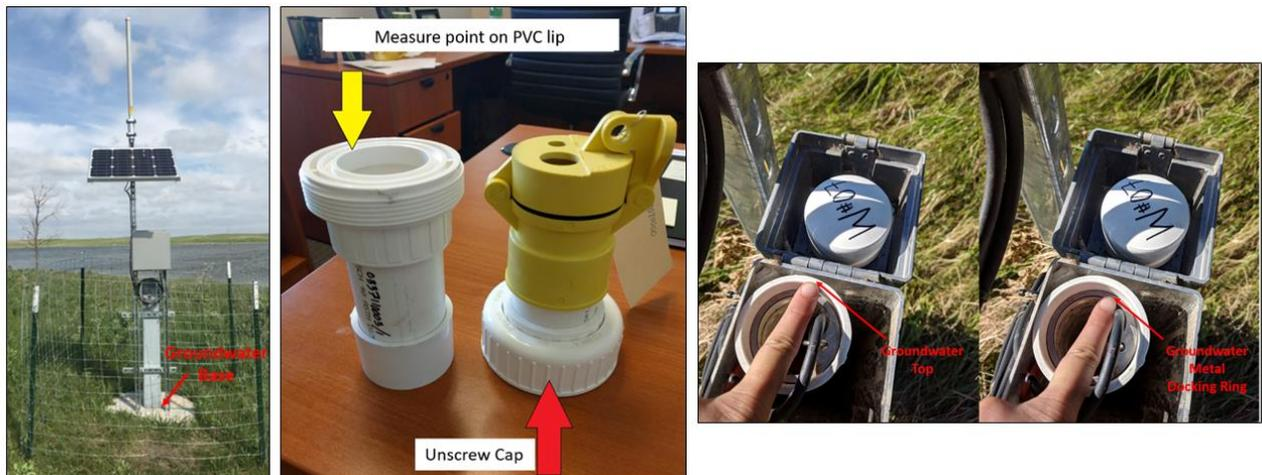
**Figure 9.** From left to right: NEON groundwater well with arrow indicating the base, where points shall be mapped on the southern-most corner; groundwater well snorkel caps, where points shall be mapped on the south side of the top of the PVC with the entire coupler and cap removed; the top of a NEON groundwater well without a snorkel cap, where points shall be mapped at the top of the PVC collar inside the well with the PVC cap removed.
