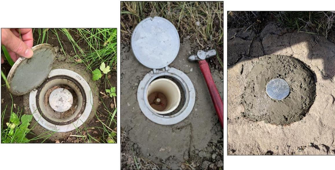
**Figure 8.** Examples of different permanent benchmark installations at NEON Aquatic sites. From left to right: round monument style benchmark with a triangle divot within a hinged access cap; datum point style benchmark within a hinged access cap; round monument style benchmark installed directly in bedrock.
