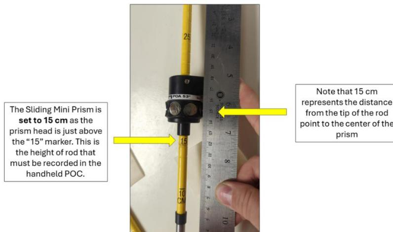
**Figure 18.** Assessing the height of rod on the Sliding Mini Prism.
