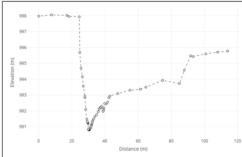
**Figure 12.** Example of high-resolution cross-section survey data where the floodplains, banks, and active channel are well-characterized by properly spaced points (each dot represents a mapped shot).
