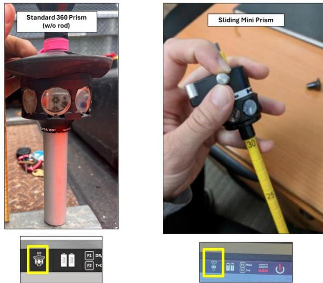
**Figure 17.** The two different prism types used for NEON total station surveys with images below that indicate which prism is selected on the POC screen.
