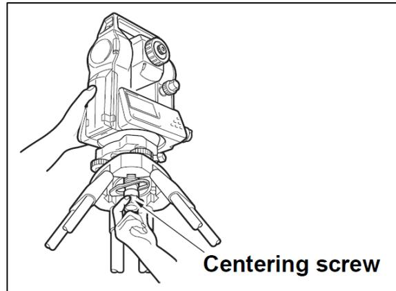
**Figure 4.** Attaching the Total Station head to the top of the tripod.
