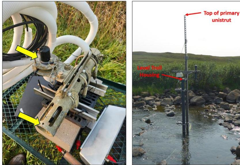
**Figure 14.** Left: Cinder block littoral station design with the yellow arrows indicating the locations on the TROLL housing and PAR sensor where points are to be mapped (the vertical pipe is not shown but this location also requires a mapped point); Right: standard littoral station design with the red arrows indicating the top of the primary unistrut and the top of the PVC cap, the latter of which is to be removed so that point is mapped on the lip of the PVC.
