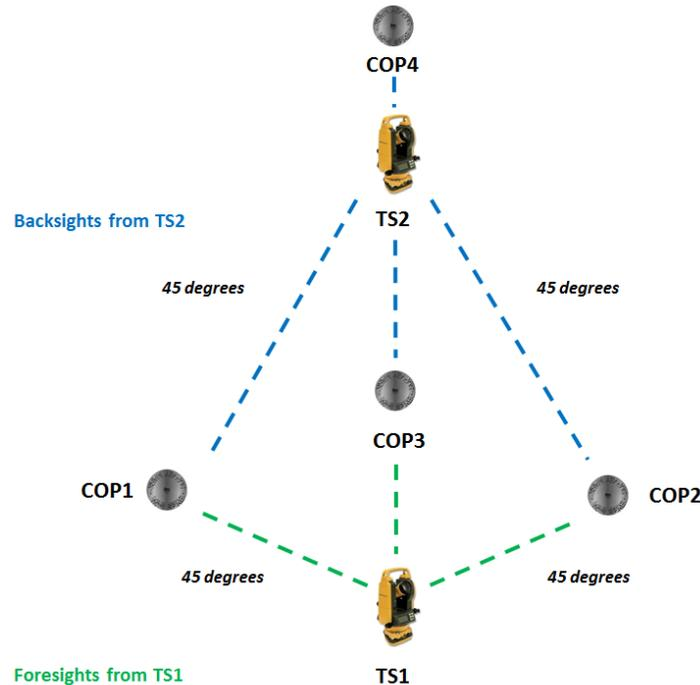
**Figure 7.** Ideal total station-control point setup using an optional fourth control point to set a second total station location (TS2). Note the wide 45-degree angles between COP1 and COP2, how COP4 is beyond TS2 and how the foresight is shorter than the backsight.
