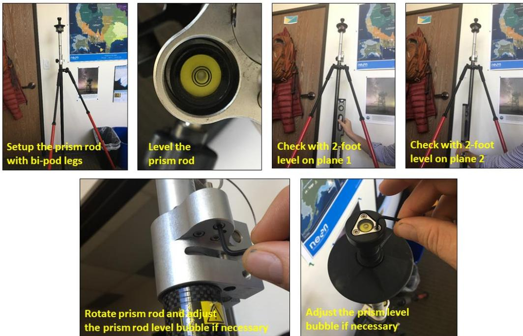
**Figure 2.** Calibrating the prism rod and prism head. A one-foot or two-foot level may be used to check the level of the prism rod.
