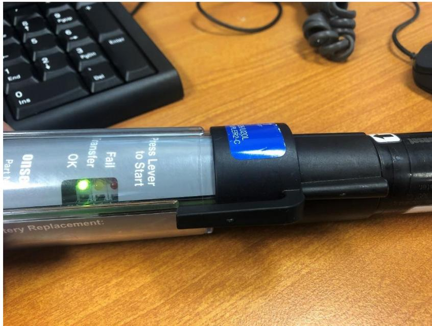
**Figure 2.** A green light indicates a successful data transfer from the logger to the shuttle after pressing the lever to start the transfer.
