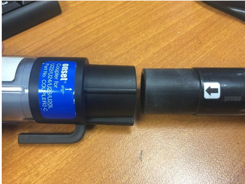
**Figure 1.** Plug a HOBO U24 logger into the shuttle with the coupler attached. Ensure proper alignment. This is ideally performed while the shuttle is connected to a laptop with HOBOWare Pro installed so that you can re-sync the logger's time in UTC (GMT).
