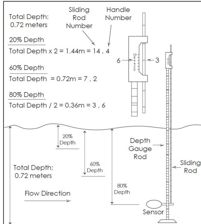
Figure 4. Correctly-assembled wading rod adjusted to 80%
