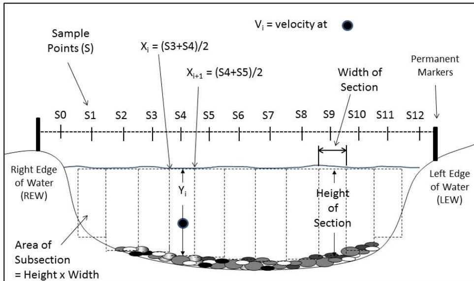
**Figure 8.** Components for manual discharge calculation
