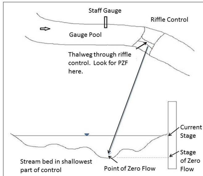
Figure 10. Diagram showing point of zero flow and stage of zero flow
