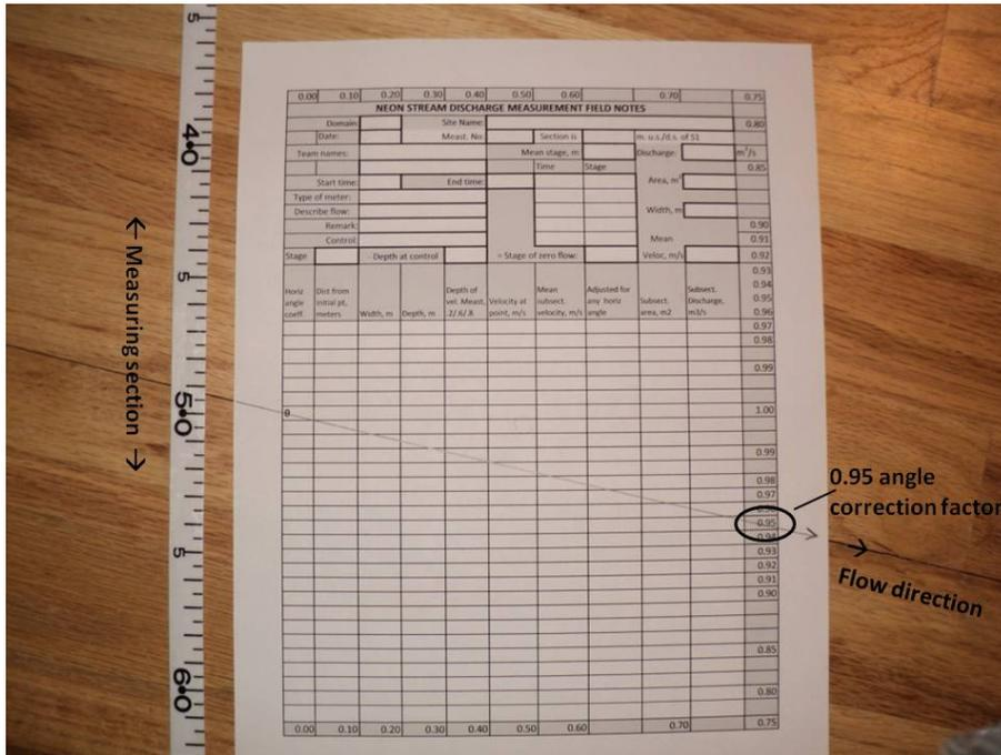
**Figure 11.** Example of correction for non-perpendicular flow using the data sheet in Appendix G
