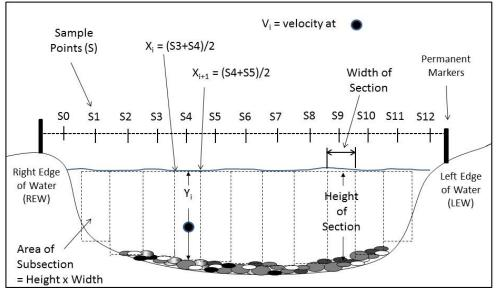
Figure 8. Components for manual discharge calculation
