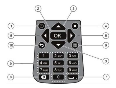
Figure 12. Keypad layout for the Hach FH950 portable flowmeter
