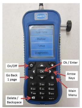
Figure 6. Hach FH950 velocity-meter showing the "Start" menu
