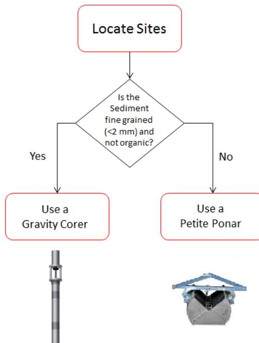
**Figure 3.** Decision flow chart 2 for determining appropriate sampler to use in the field
