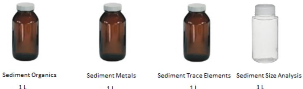
**Figure 5.** Example of Amber bottles used for collecting organics, metals and trace elements and a Teflon bottle for sediment size samples
