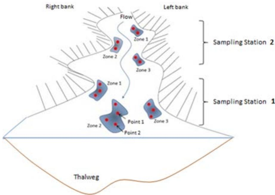
**Figure 1.** Identifying the location for sediment sampling in non-wadeable streams. The two sediment sampling stations should contain depositional zones that represent upstream influences and various flow regimes; left bank (looking downstream), right bank ((looking downstream), central channel, and different depths of water
