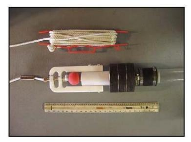
Figure 9. Gravity corer sampler for use in lakes and non-wadeable streams
