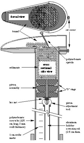
Figure 10. Set-up for sediment sub-sectioning and extrusion (from EPA, 2012)
