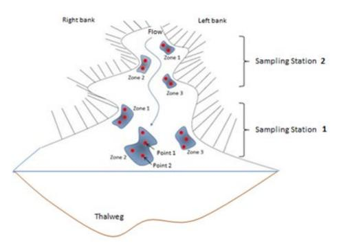
**Figure 1.** Identifying the location for sediment sampling in non-wadeable streams. The two sediment sampling stations should contain depositional zones that represent upstream influences and various flow regimes; left bank (looking downstream), right bank ((looking downstream), central channel, and different depths of water
