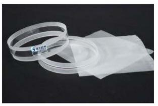
Figure 11. Sieve mesh and sieve frame for sediment sample processing
