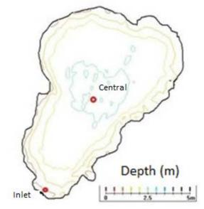
**Figure 6**. Identifying the Station for sediment sampling in lakes. The two sampling Stations (red circles) should denote depositional zones in the center of the lake (deepest section) and in a nearshore depositional environment
