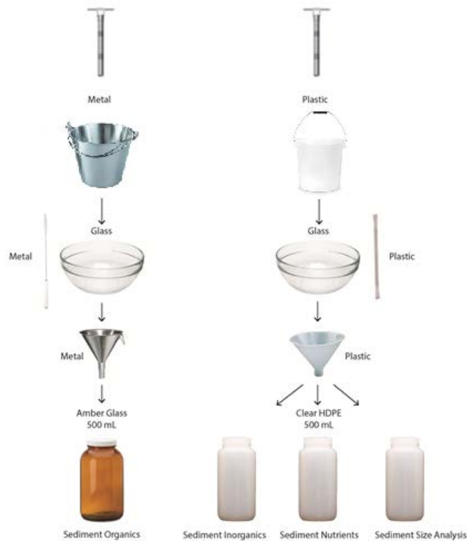
Figure 11. Sediment collection instruments by sample type
