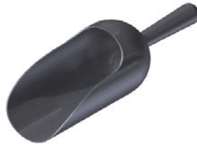
Figure 12. Scoop sampler for use in wadeable streams
