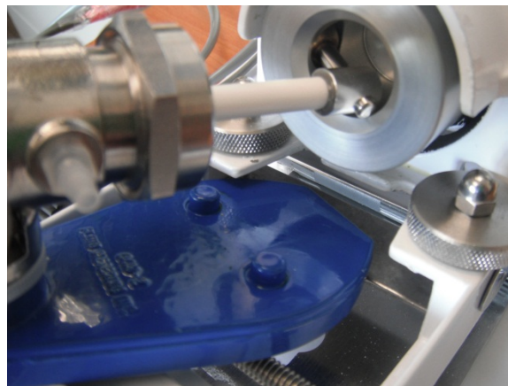
Figure 1. Fluid metering pump a) Components of pump drive (left) and pump head (right), b) Configuration of pump head (modified from fluidmetering.com/materials-construction.html ), and c) Assembly of pump head into pump drive
