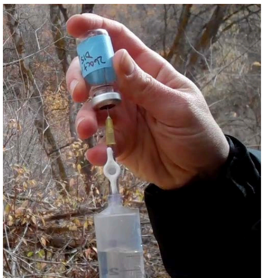
Figure 11. Insertion of the needle into the gas vial through the rubber septum
