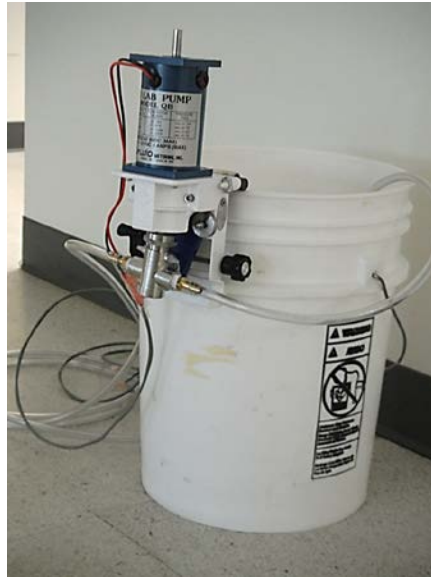
Figure 5. Mounting of the pump on the conservative tracer bucket
