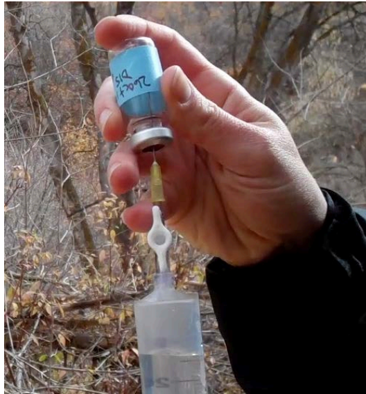
Figure 12. Insertion of the needle into a gas vial through the rubber septum. Note: Actual gas vials used by NEON may look different than in the picture
