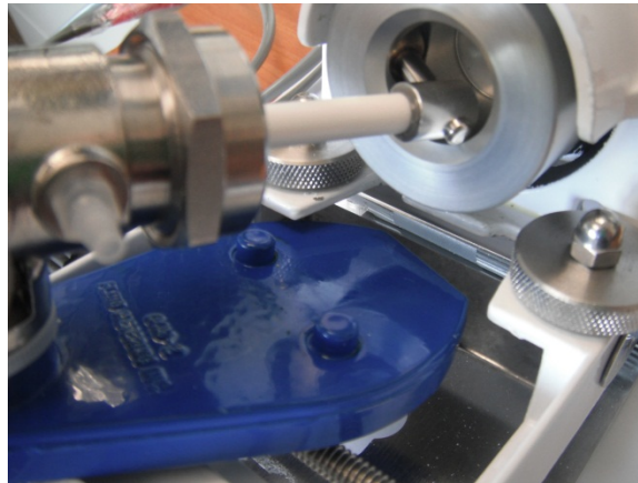
Figure 14. Fluid metering pump a) Components of pump drive (left) and pump head (right), b) Configuration of pump head (modified from fluidmetering.com/materials-construction.html ), and c) Assembly of pump head into pump drive
