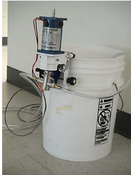
Figure 6. Mounting of the pump on the conservative tracer bucket
