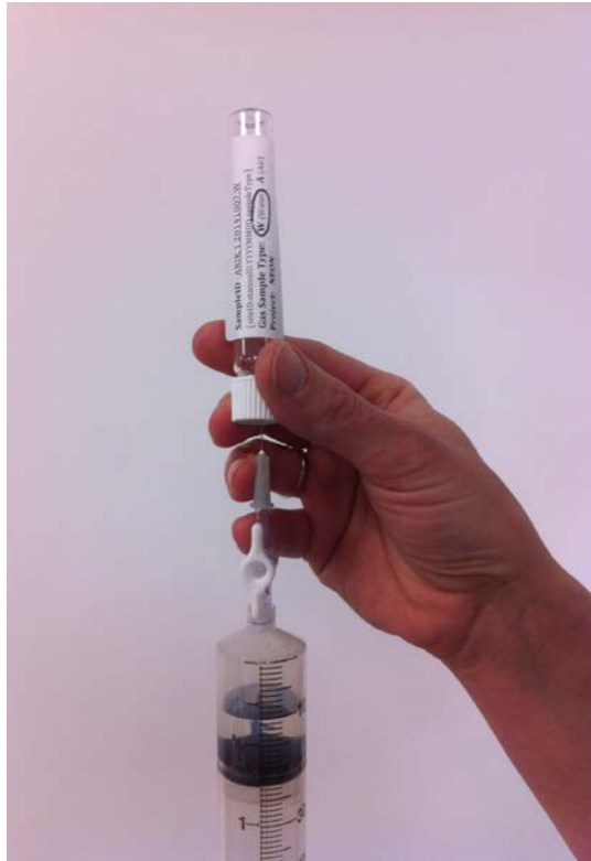
Figure 12. Insertion of the needle into a gas vial through the rubber septum.
