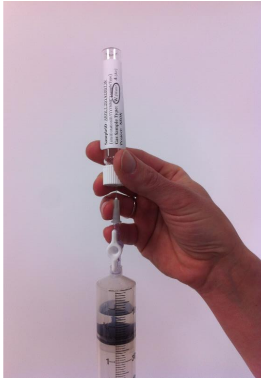
Figure 12. Insertion of the needle into a gas vial through the rubber septum.
