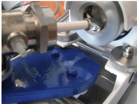
**Figure 16.** Fluid metering pump a) Components of pump drive (left) and pump head (right), b) Configuration of pump head (modified from [fluidmetering.com/materials-construction.html](http://fluidmetering.com/materials-construction.html)), and c) Assembly of pump head into pump drive
