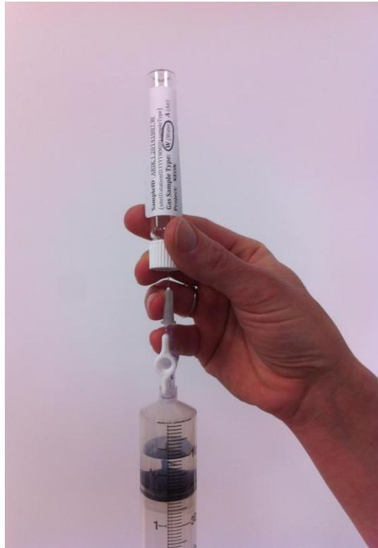
**Figure 13.** Insertion of the needle into a gas vial through the rubber septum.
