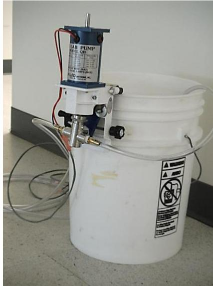
**Figure 7.** Mounting of the pump on the conservative tracer bucket
