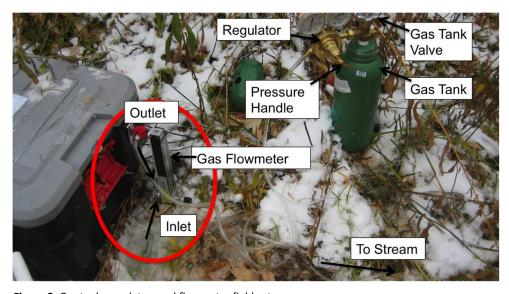
Figure 8. Gas tank, regulator, and flowmeter field setup
