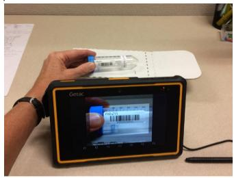
Figure 14. Barcode label scanning.
