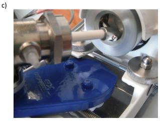
**Figure 16.** Fluid metering pump a) Components of pump drive (left) and pump head (right), b) Configuration of pump head (modified from fluidmetering.com/materials-construction.html), and c) Assembly of pump head into pump drive
