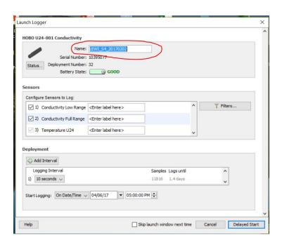
f) Before disconnecting HOBO check that shuttle was powered on while launching and you can check the HOBO status in HOBOware Pro before disconnecting and this will show you if it is
