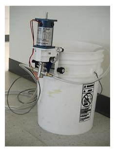
**Figure 7.** Mounting of the pump on the conservative tracer bucket
