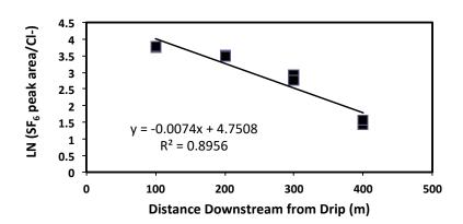
Figure 15. Example SF6 loss rate data calculation.
