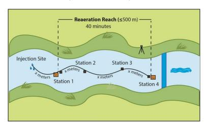
**Figure 5.** Schematic of stream reach with injection site and four downstream sampling stations. Travel time between Station 1 and 4 should be  $\sim$ 40 minutes. Note that Reaeration station 1 is co-located with Sensor set 1 and Reaeration station 4 is co-located with sensor set 2.
