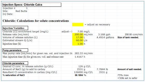
Figure 3. Example of injection calculation worksheet. Modified from LINX II.
