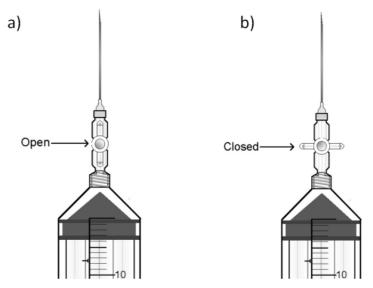
Figure 12. Example of a syringe with a stopcock with attached needles in the a) "open" and b) "closed" positions
