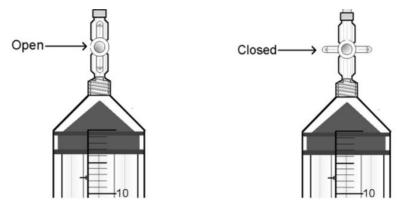
Figure 9. Example of a syringe and stopcock in the "open" and "closed" positions
