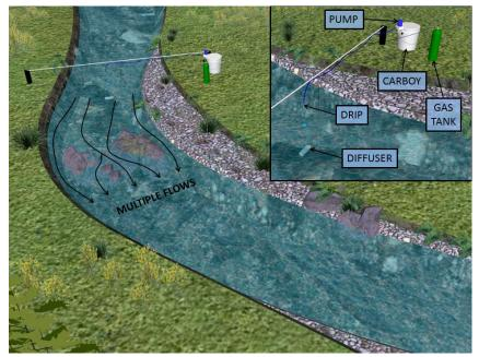
Figure 6. Field setup of the injection site with conservative tracer and inert gas
