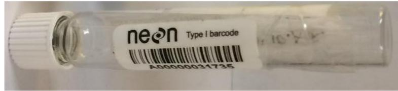
Figure 5. Example of tracer gas vial labels.
