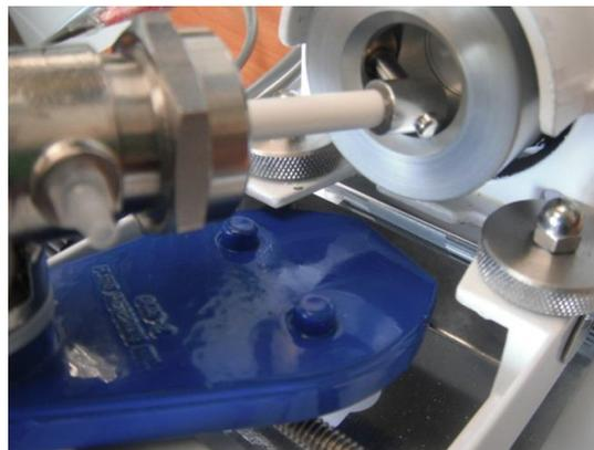
**Figure 19.** Fluid metering pump a) Components of pump drive (left) and pump head (right), b) Configuration of pump head (modified from [fluidmetering.com/materials-construction.html](http://fluidmetering.com/materials-construction.html)), and c) Assembly of pump head into pump drive
