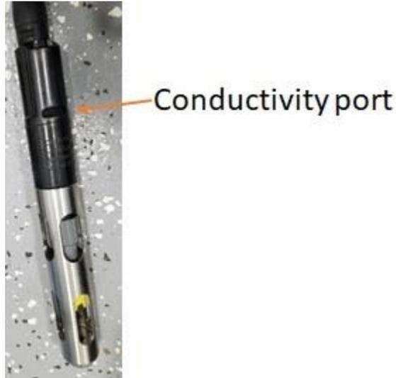
**Figure 6.** Conductivity sensor is located at the top of the probe. Ensure the entire probe is in the water for accurate readings.
