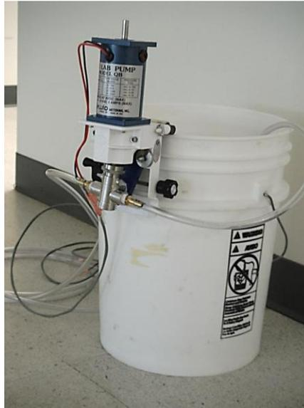
**Figure 9.** Mounting of the pump on the conservative tracer bucket
