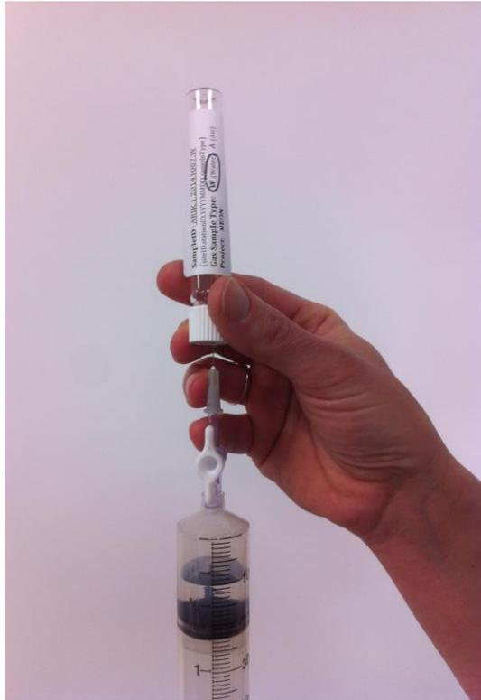
**Figure 15.** Insertion of the needle into a gas vial through the rubber septum.
