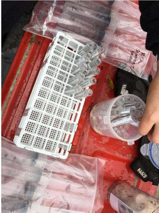
**Figure 4.** vialID number written on the bottom of each vial to help locate vials quickly.
