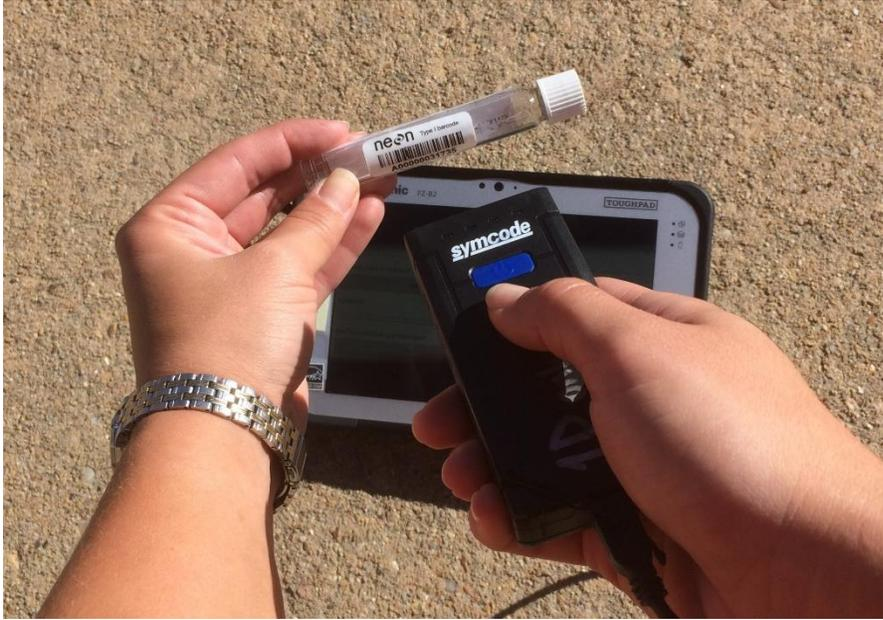
**Figure 16.** Barcode label scanning.
