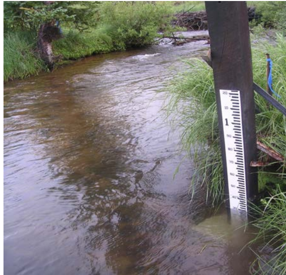
Figure 6. Example of staff gauge installed in a pool
