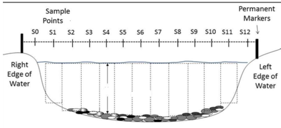
Figure 2. Example of an excellent distribution of measurement section
