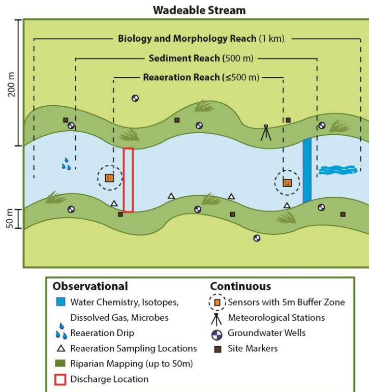
Figure 1. Discharge station must be placed on a run or riffle associated with the pool that the staff gauge and pressure transducer is placed.
