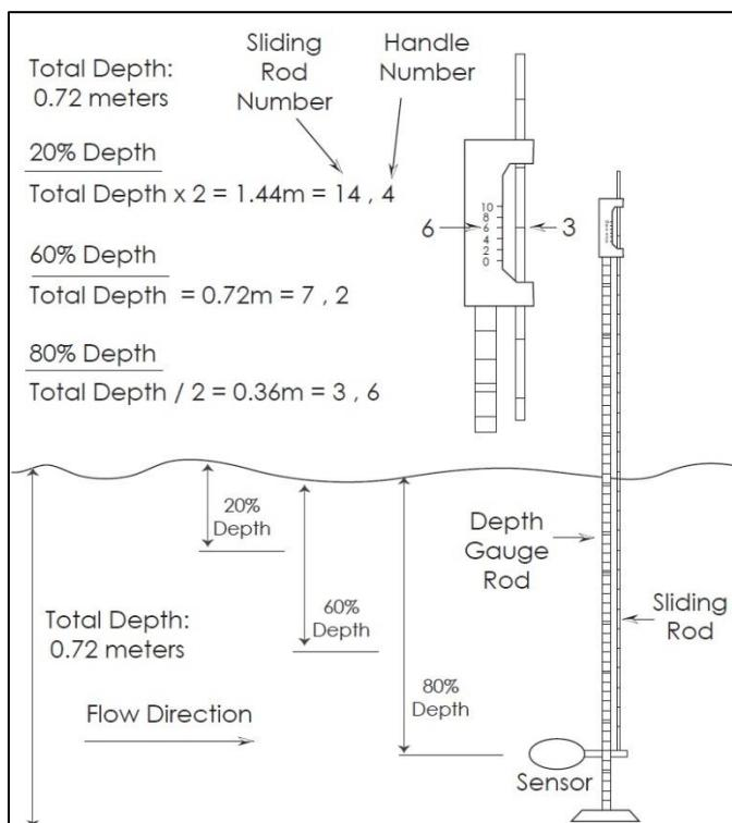
Figure 4. Correctly, assembled wading rod adjusted to 20, 60, and 80%
