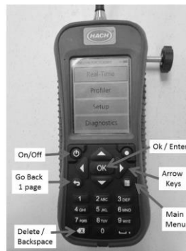
Figure 3. Hach FH950 velocity meter showing the “Start” menu.
