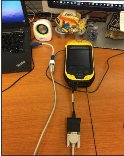
**Figure 12. Proper setup of the Trimble receiver using the three serial cables connected together. Note that the Tornado antennae is not attached in this example.**
