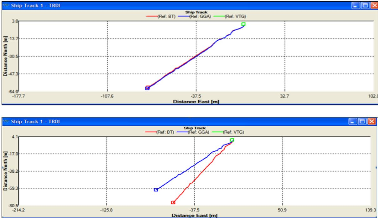
**Figure 13. Above: Proper compass calibration and Magnetic Variation coupled with good GPS data – lines are in agreement. Below: Poor compass calibration and/or Magnetic Variation is not set correctly. Lines are not in agreement. Check calibration, Magnetic Variation value, and potential Moving Bed conditions. Check GPS coverage, latency, and satellite conditions.**
