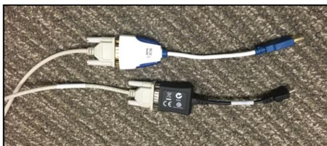
**Figure 10. Trimble to PC connection serial cables. This set contains three cables that must be attached: the Trimble to 9-pin (male); the 9-pin (female) to 9-pin (female); and the RS-232 9-pin (male) to USB.**
