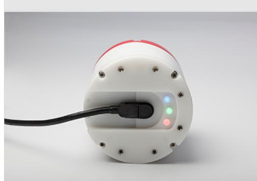
**Figure 36.** RiverPro ADCP. Left: base of the ADCP showing the five beam lenses; Right: top of the ADCP with indicator lights and power cord.
