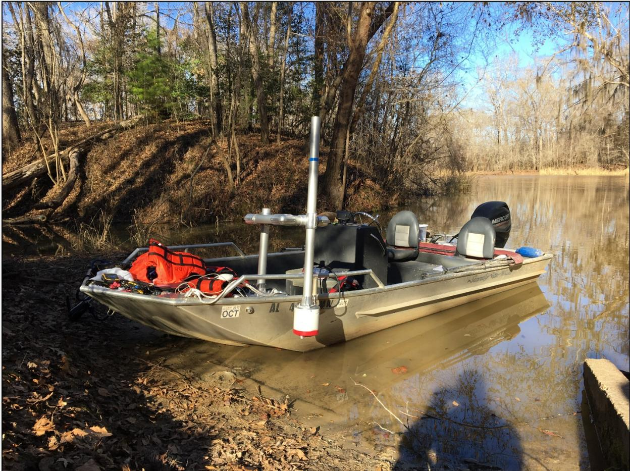
**Figure 62.** The Kentucky II mount (USGS) is used to deploy the ADCP when measuring discharge at NEON river sites using the piloted boat method.
