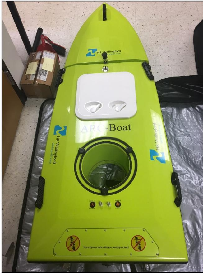
**Figure 37.** The ARC-Boat is the preferred deployment method to measure discharge at NEON river sites.
