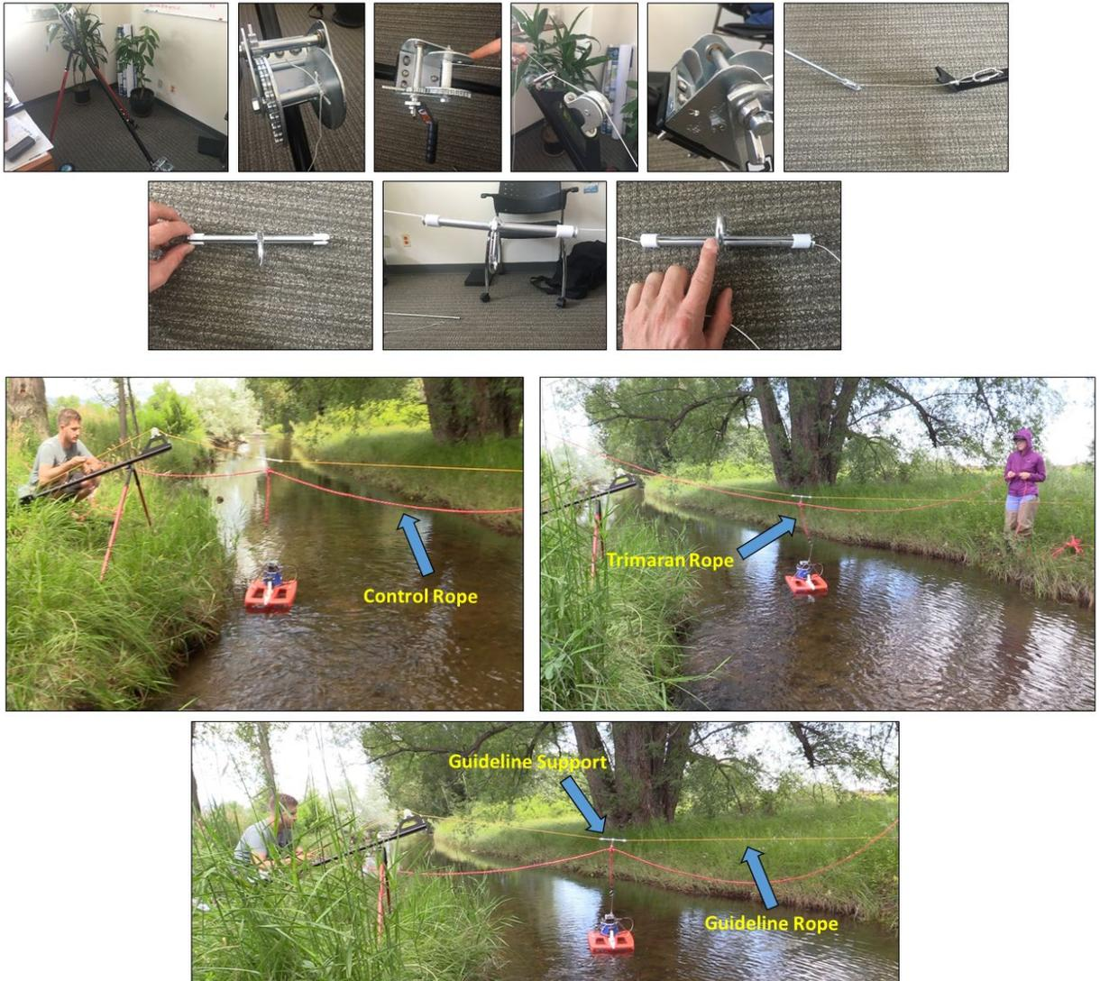
Figure 21. Assembling the Temporary High Line.
