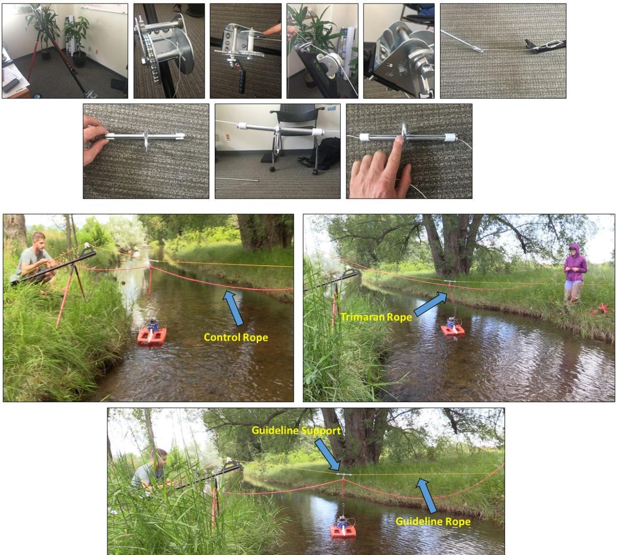
**Figure 21.** Assembling the Temporary High Line.
