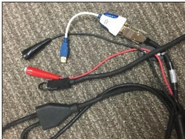
**Figure 63.** Serial cables that connect the ADCP to the 12V battery and the laptop PC. Note the white RS-232 USB adapter that must be included in the set.
