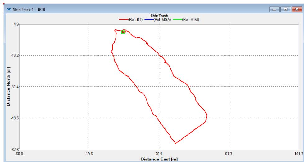
**Figure 51.** The WinRiver II Ship Track window observed during a loop moving bed test. The green box indicates the boat starting position, the line shows the boat path as it is navigating across the channel and turned back around toward the starting bank, and the red box indicates the boat ending position.
