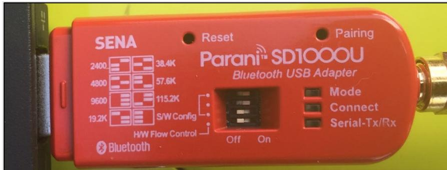
**Figure 17.** Top: Parani-SD1000U USB Bluetooth Adapter with default settings. Bottom: Correct settings for ADCP and GPS Bluetooth configuration.
