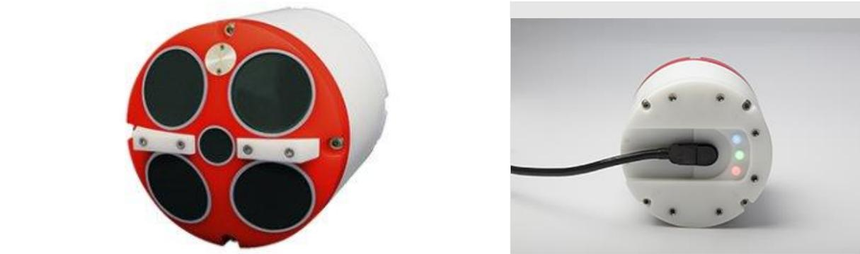
**Figure 36.** RiverPro ADCP. Left: base of the ADCP showing the five beam lenses; Right: top of the ADCP with indicator lights and power cord.
