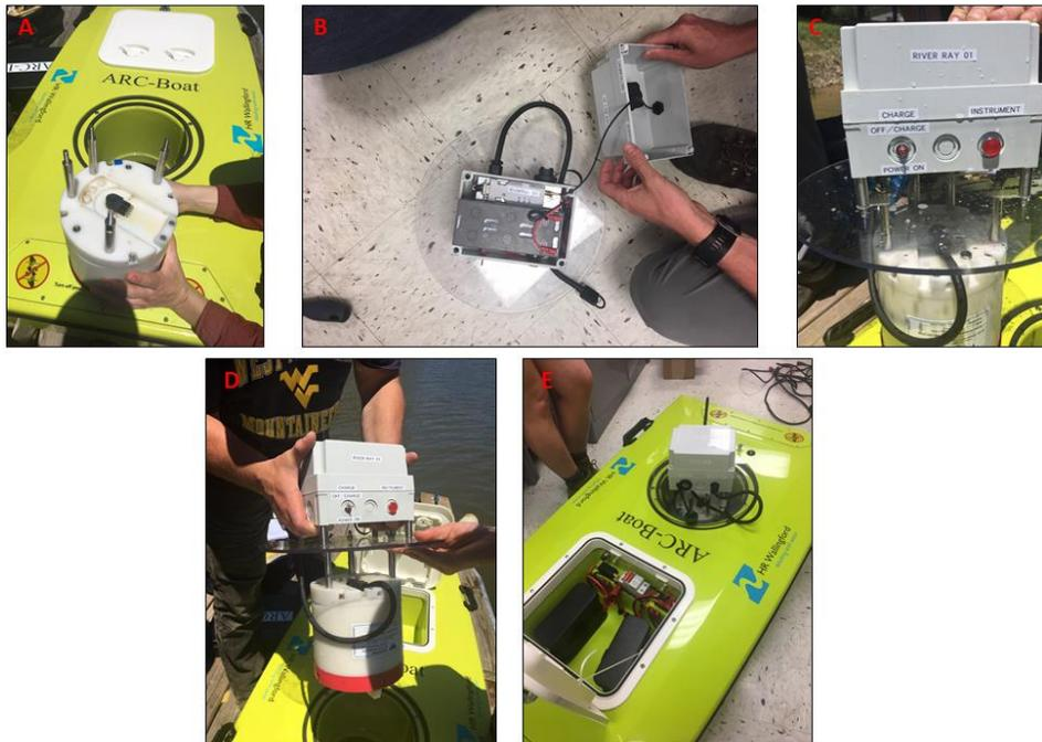
**Figure 38.** The ARC-Boat setup with the RiverPro ADCP adapter. A: connect the long set screws to the top of the ADCP; B: connect a fully charged 12V battery inside the ADCP adapter; C: connect the long set screws to the circular base plate of the adapter with the wingnuts, connect the ADCP cable coming out of the adapter to the
